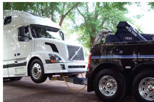
Miller Industries has designed the latest innovation in lift fork technology. The forks are cast in steel alloy, that weighs half as much as a conventional welded style lift fork. Available only through Miller Industries Distributors.
