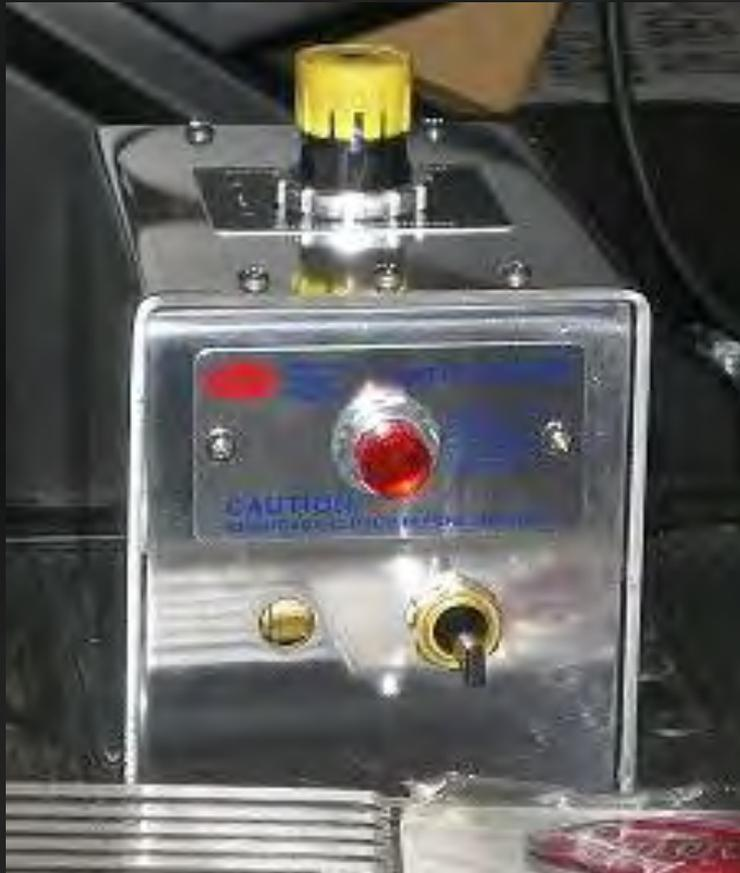
Allows for manual PTO engagement if there is an electrical failure.
