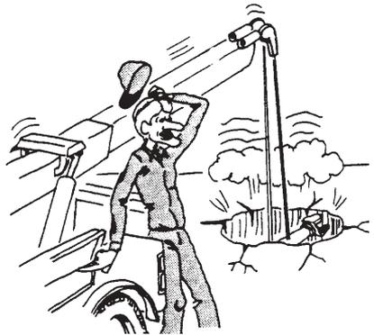
Don't disengage the winch drum clutch while the winch cable is loaded.
