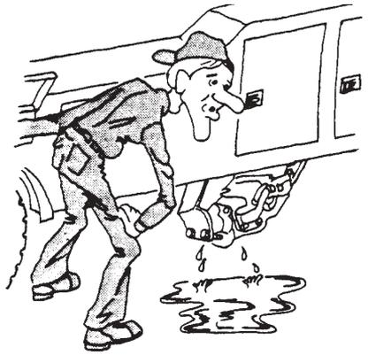
Don't operate your wrecker's engine faster than recommended. Excessive speeds can damage PTO shafts, hydraulic pumps and winches.
