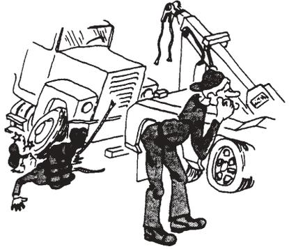
Don't exceed WORKING LIMIT ratings of cable. Use breaking strength ratings only for selecting replacement cable.
