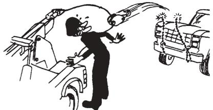
After rigging cables, don't begin pulling without rechecking connections. Make sure that all cables and snatch blocks are securely attached and cannot accidentally pull loose.
