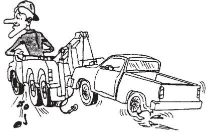
After you have hooked up a vehicle for towing, don't start the tow until you have double checked the hook-up, installed safety chains and released the parking brakes on the towed vehicle.
