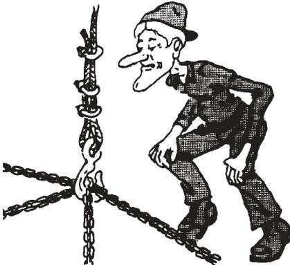
Don't use winch cables with hooks attached by means of cable clips. Use only cables with hooks attached by means of thimbles and machine swaged terminals.
