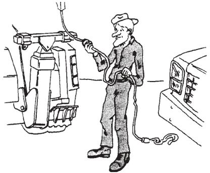
Don't use damaged cables on your wrecker. Become familiar with the various types of cable damage and carefully inspect all cables being used in a recovery operation before starting to pull.
