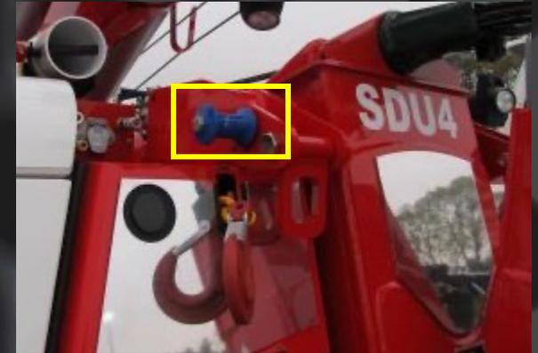
Allows for quicker retrieval and return of safety chains into the safety chain pockets
