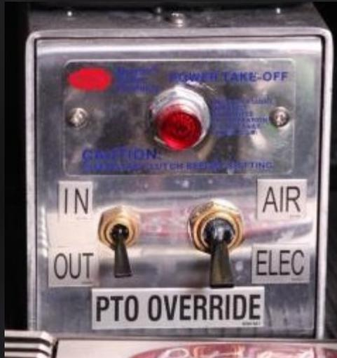
Allows for manual PTO engagement if there is an electrical failure.
