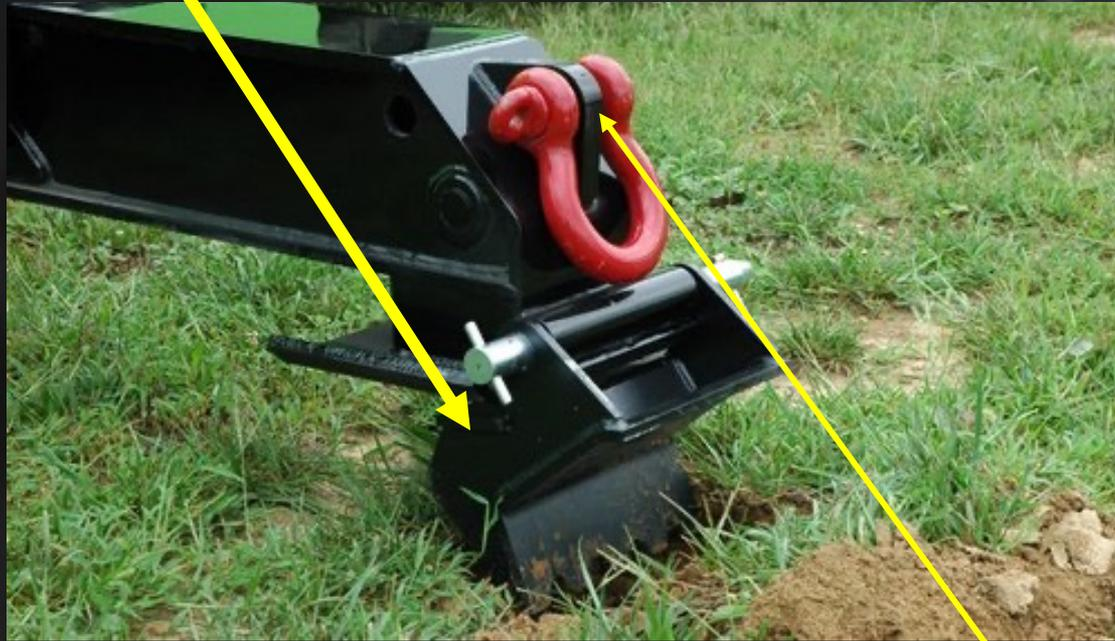
Note Product Feature of H-Beam Low Outriggers, Standard Tieback Lug for Screw-Pin Shackle
