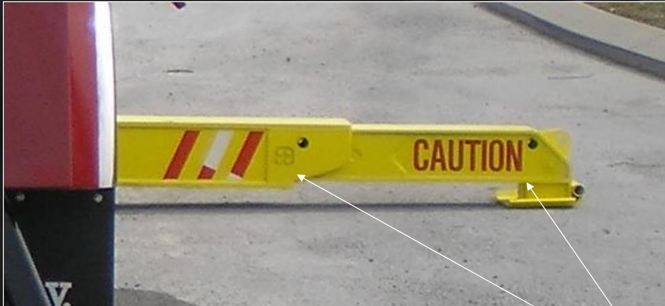
Note holes that allow legs to be pinned fully in or out during a side pull
