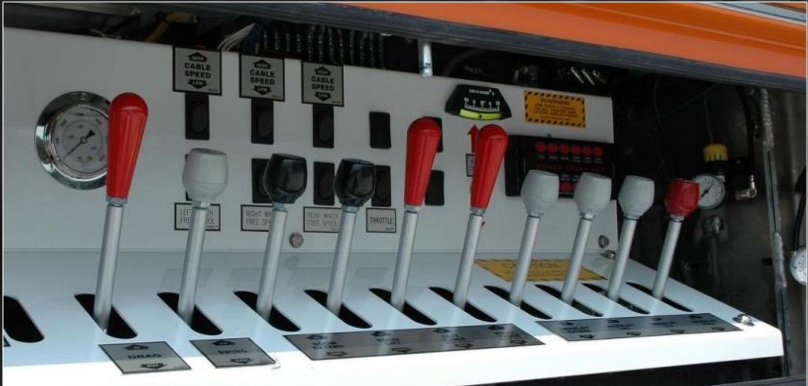
Allows for a maximum of 1 deck drag winch. Not available with two or more auxiliary winches. Includes manual control handles for all outriggers
