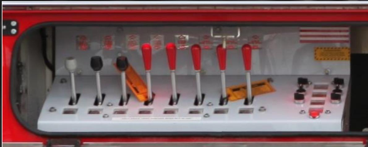
This option adds manual controls to the passenger side and replaces the panels as shown on the lower right of the previous slide.
