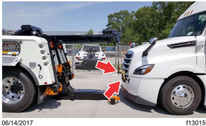
Fig. 10, Tow Cables Connected to the Tow Hooks
