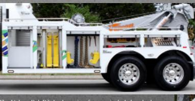
The Vulcan PolyBilt body option features include brushed aluminum roll-up doors with remote lock/unlock, adjustable poly shelving, chain racks lift fork storage.
