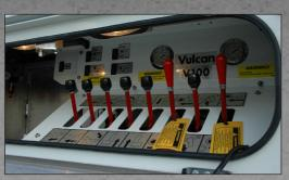
Illuminated manual controls, winch air-free spools, and pressure gauges are standard on the drivers & passenger side control stations.
