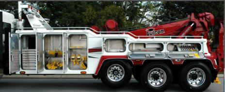
The newly designed aluminum body provides spacious, modular tool compartments with features that include keyless entry, washable floors, adjustable shelves, rear tailboard fork storage, along with chain racks and fork holders. Other popular options include a 7-drawer tool box, and fold-down storage brackets for the heavy-duty tire lift.
