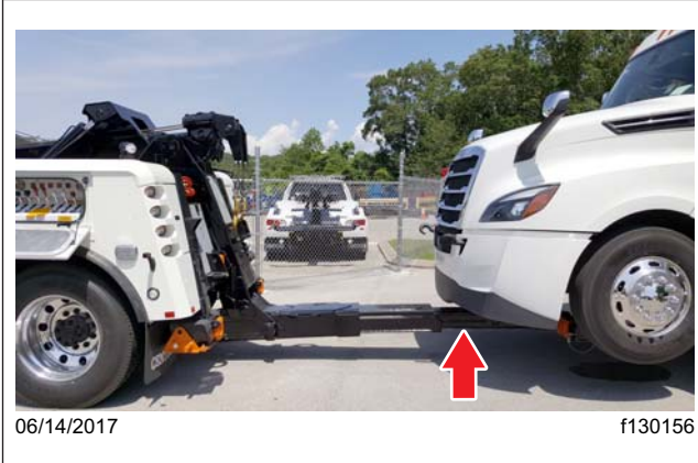
Fig. 11, Retracting the Recovery Boom
