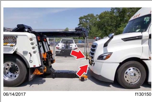
Fig. 5, Tow Cables Connected to the Tow Hooks
