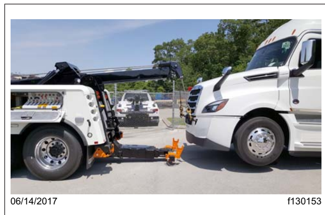
Fig. 8, Backing the Tow Truck with Lift Adaptors on the Crossbar
