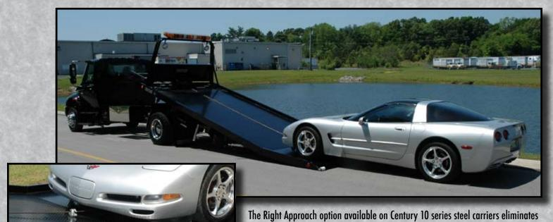
the need for wood planks or ramps when loading and unloading low clearance vehicles. The release handle allows the rear hinged deck section to be lowered to a 6° load angle. A cable guide is inserted in the deck to keep the cable low while winching the vehicle onto the rear deck.
