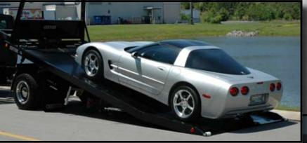
After the vehicles front wheels are on the carrier, the deck can be leveled out and the cable guide removed allowing the vehicle to overcome the second clearance problem with the forward section of the deck. With the front wheels on the front section of the deck the process can be repeated again to eliminate clearance problems such as low exhaust or extended rear overhang
