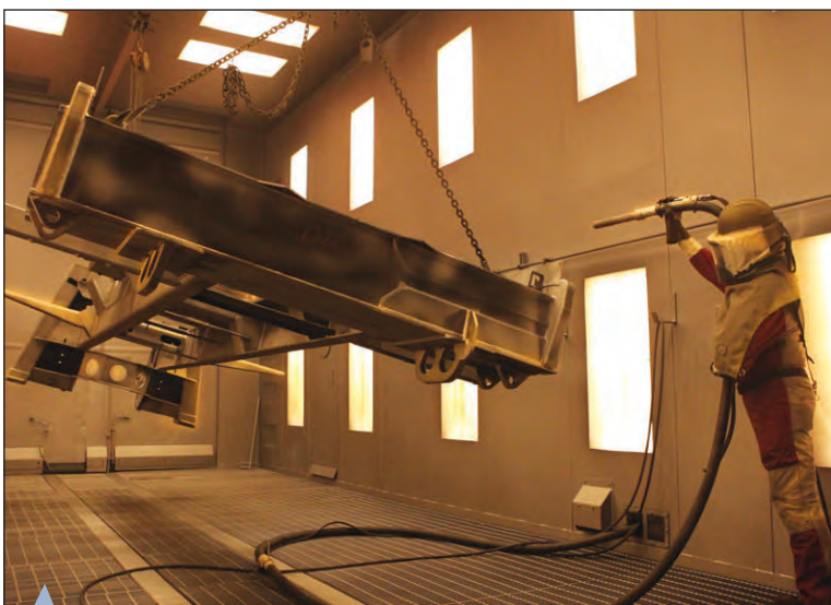
In addition to the two media blast booths in Ooltewah, additional booths have been added to the Greenville, Tenn. and Hermitage, Penn. facilities with an additional booth under construction in Mercer, Penn. This cleaning process removes any rust, oil or imperfections in the metal to provide higher-quality surface for primer and paint adhesion.
