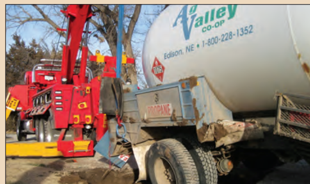
The Century 5130 was rigged to stabilize the vehicle as the rotator lifted the rear.
