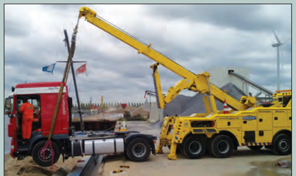
The Century 9055 lifts the front of the loaded trailer clear of the tractor.
