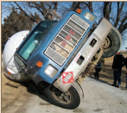
The Century 5130 was rigged to stabilize the vehicle as the rotator lifted the rear.
