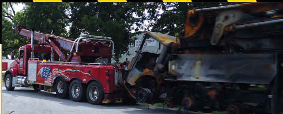
The boom of the 1075S was swung forward to provide additional front axle weight.
