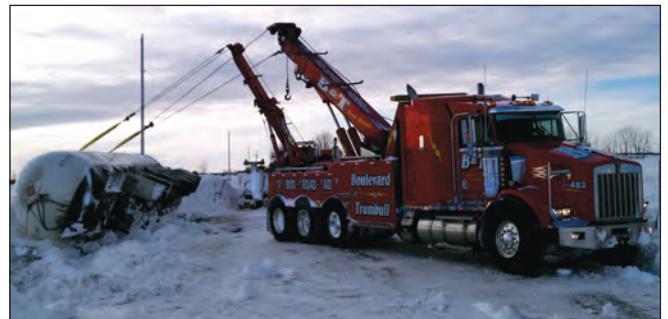
The two Century units work together to right the partially loaded tanker.
