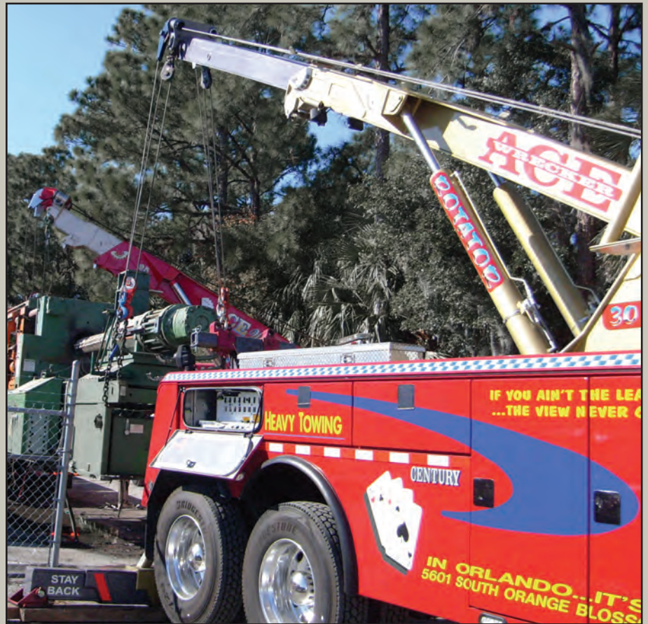
The Century 1130 makes a great second unit to work alongside another heavy-duty rotator in a wide variety of recoveries or lifting operations such as loading heavy equipment or machinery.
