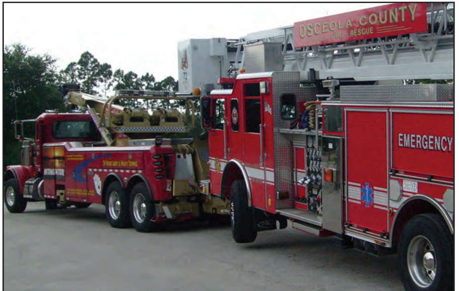
With the ability to rotate the boom forward over the cab, the operator can increase the front axle weight on his 1130 when towing heavier loads. This is especially helpful when towing those difficult snorkel, fire and bucket trucks because you can retract your underlift in closer to the back of your unit and let the towed vehicle's boom or bucket hang over the top of your unit.
