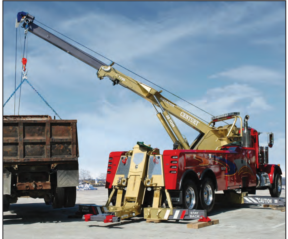
The Century 1130 has a maximum hook height of 354 inches along with a boom capacity of 60,000 lbs. retracted and 25,000 lbs. extended, making it capable of handling a wide range of vehicles and equipment.
