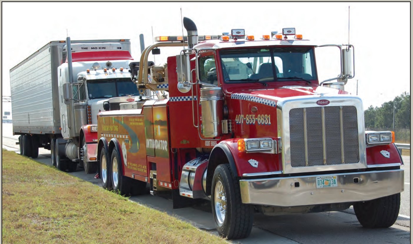
Designed to be an economical-yet-versatile unit for daily operation, the Century 1130 is ideal for both recovery and towing applications. The underlift has a 15,000-lb. lift capacity at full extension of 130 inches and towing capacity up to 80,000 lbs.
