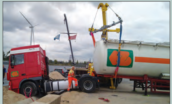
The Century 9055 lifts the front of the loaded trailer clear of the tractor.
