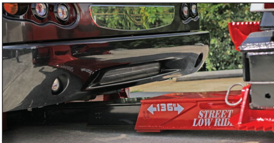
The Street Low Rider with its low profile, fabricated stinger easily gets under difficult-to-tow vehicles with room to spare.
