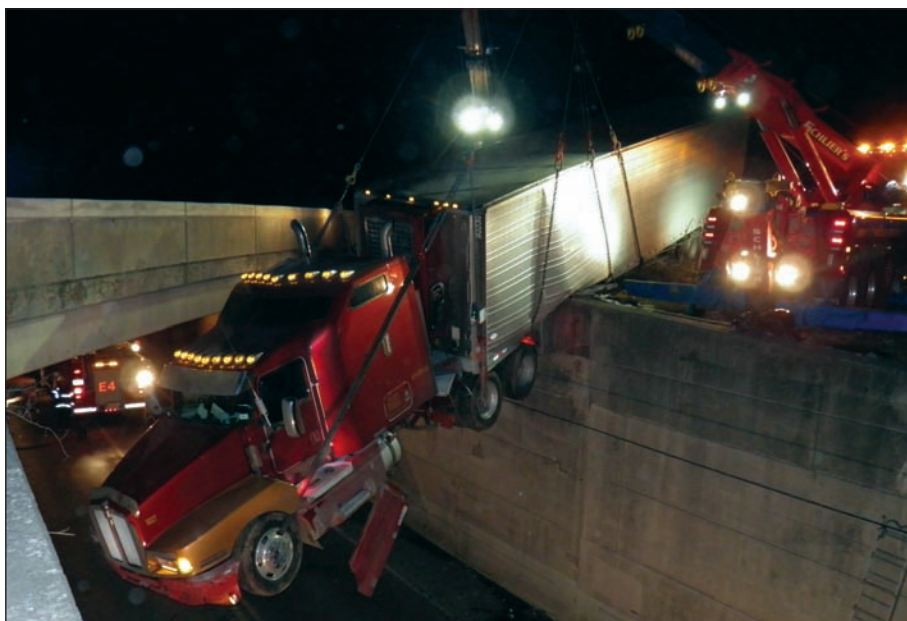
The two rotators positioned on each side of the trailer delicately lifted the tractor and front of the trailer.
