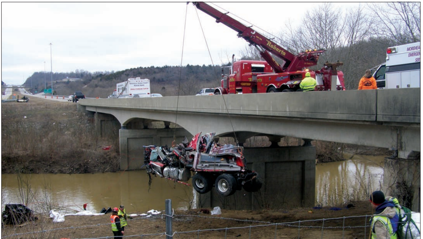
After recovering the tractor from the creek, the cab and other pieces were loaded on the chassis before lifting it back onto the bridge.
