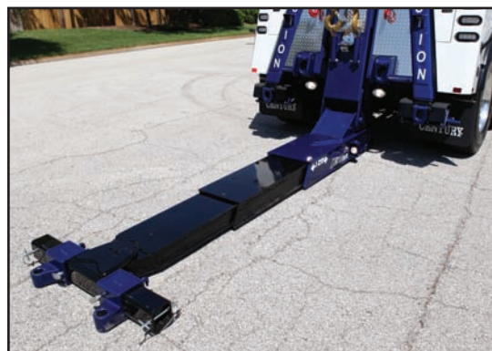
The Street Low Rider, available on the Century 7035 (pictured), 9055 and SDU-4, gives you the benefits of the low profile stinger found on the Coach Low Rider without the additional length that translates into increased overhang, heavier rear axle and lighter front axle weights on your unit. Miller offers both models, so you can choose the equipment that best fits your specific towing needs.
