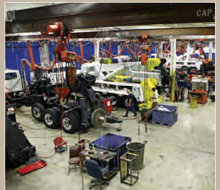
One of the heavy-duty unit's last stops at Miller is in one of 14 install bays, where it's outfitted with any additional components, lights or accessories requested by the customer.
