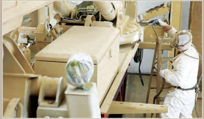
Every LBU welded component receives a thorough coating of epoxy primer before being sent to assembly.
