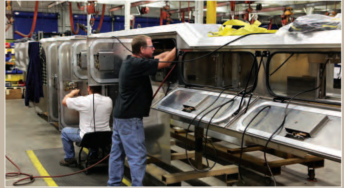
While the center section is being assembled, experienced Miller technicians mount one-piece wiring harnesses in the unit's aluminum modular toolboxes.
