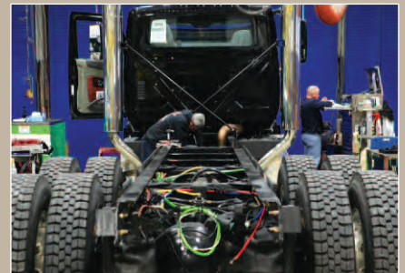
Before the center section is mounted, the chassis is prepped with the frame cut to length, mounting rails drilled and installed, and the PTO and pump installed.
