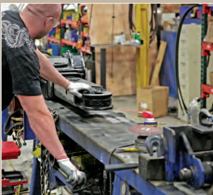
As each recovery unit is put together, it's subjected to ongoing testing throughout the assembly process to ensure that fit and operation are correct at every stage.
