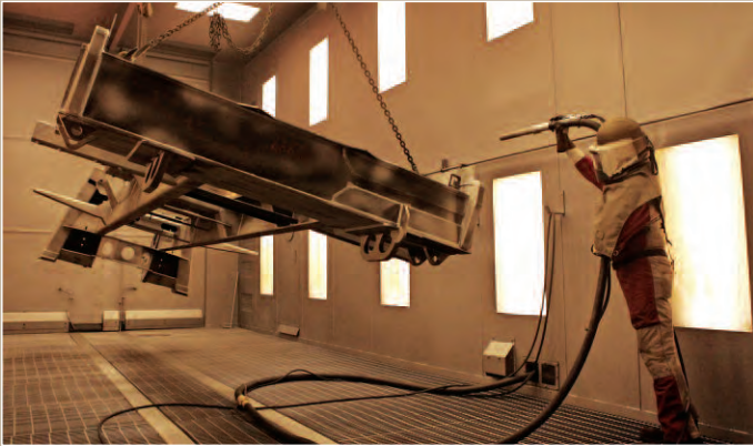
The media blast process removes any rust, oils or imperfections in the metal before the parts are transferred to the paint booth.
