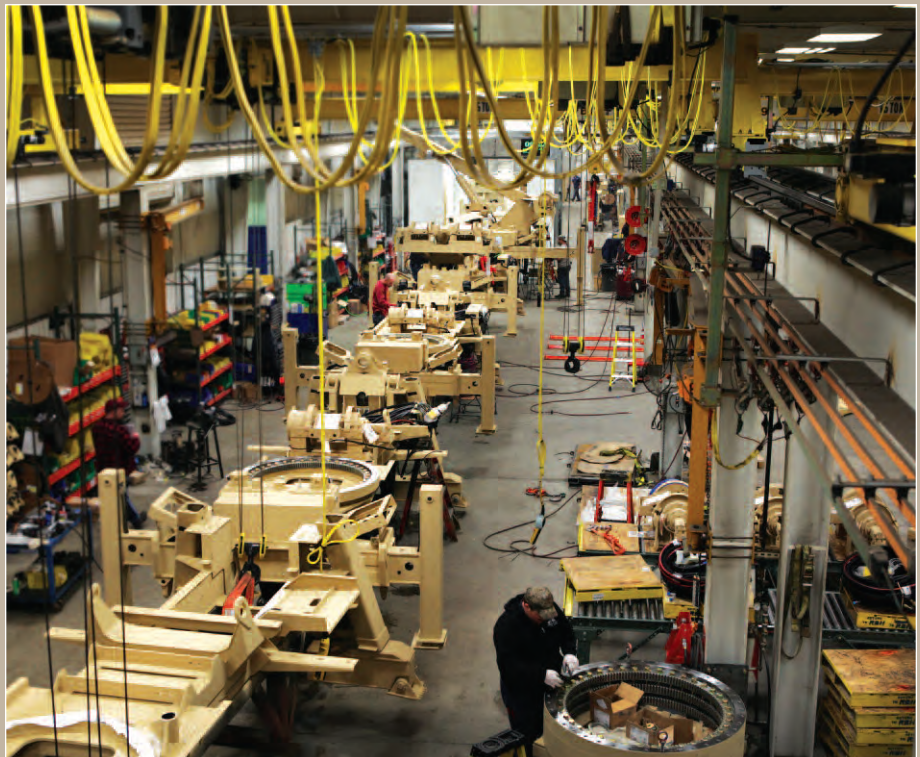
After all the welded components have been blasted and painted, they're united with the purchased components on the LBU assembly line.
