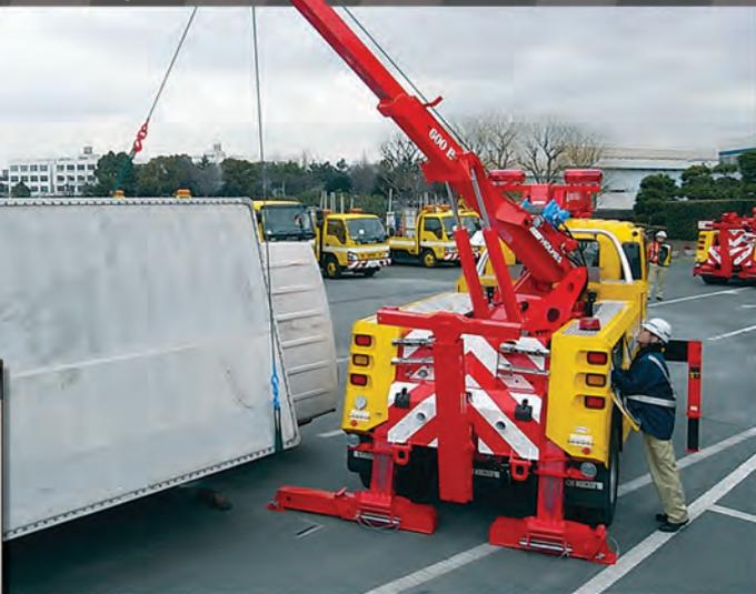
unit to assist in handling the approximately 40 accidents per day on the busy thoroughfare. Leading into Tokyo, the Expressway includes narrow, elevated roadways and long, low-ceilinged tunnels. A specially equipped Holmes 600R outfitted with an additional crane for material handling was put into service and has performed flawlessly.
