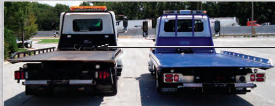
With 5 to 6 inches of lower deck height compared to a conventional carrier, the LCG provides better stability when driving down the road loaded as well as improved height clearance when hauling taller loads or operating under many lower awnings or in garages.
