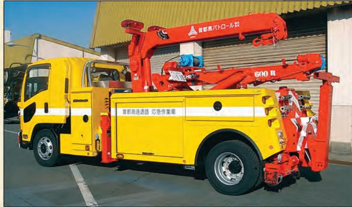
unit to assist in handling the approximately 40 accidents per day on the busy thoroughfare. Leading into Tokyo, the Expressway includes narrow, elevated roadways and long, low-ceilinged tunnels. A specially equipped Holmes 600R outfitted with an additional crane for material handling was put into service and has performed flawlessly.
