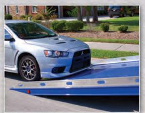
The extremely low load angle makes it ideal for loading vehicles with low spoilers, bumpers or exhaust pipes without the use of ramps or wood.
