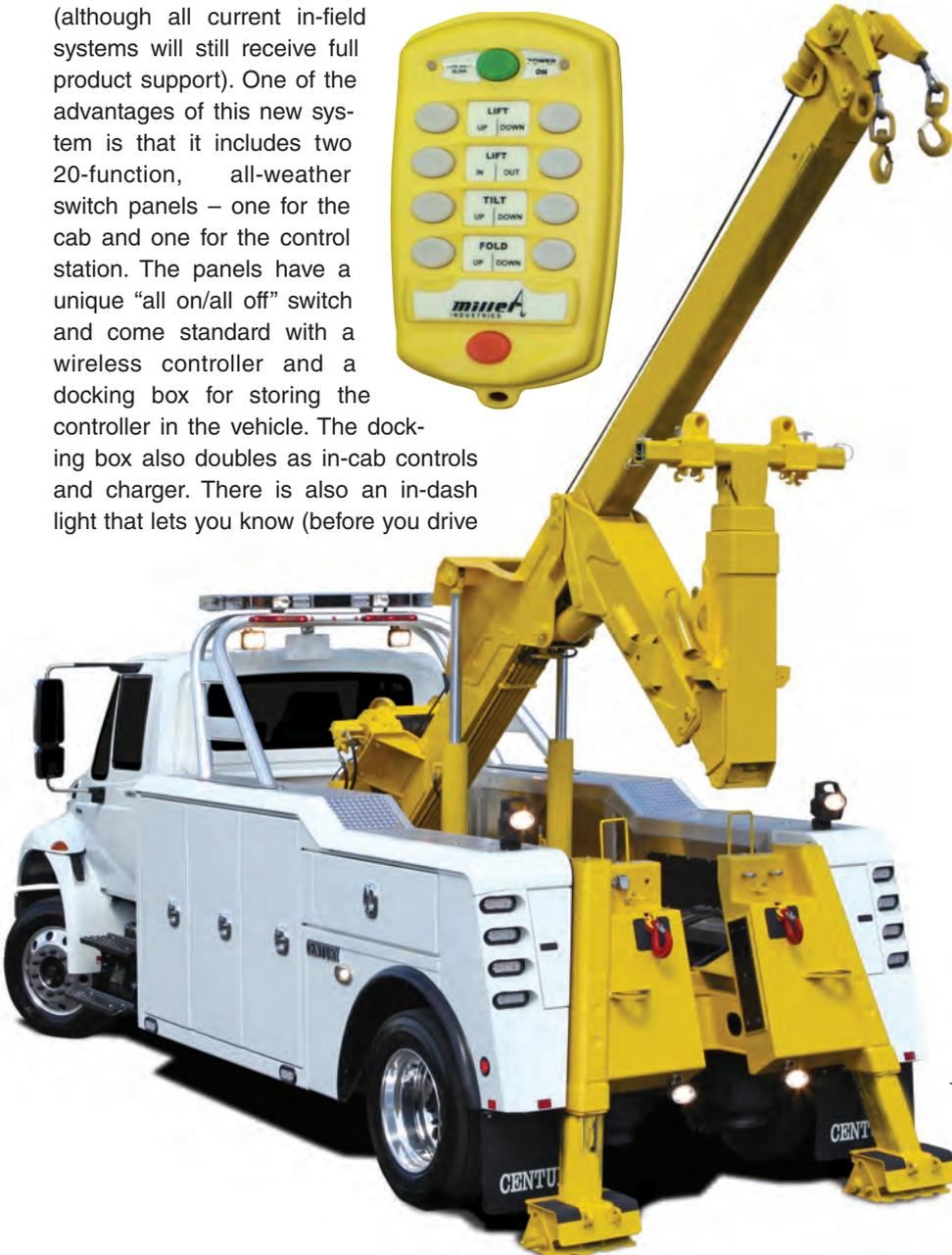
*The 4024/T2 features a new fabricated deep “U” design for the recovery boom. All new heavy-duty Miller units with the aluminum modular tool compartments feature newly designed latches that include power lock.*
