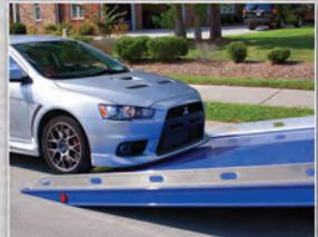
The extremely low load angle makes it ideal for loading vehicles with low spoilers, bumpers or exhaust pipes without the use of ramps or wood.
