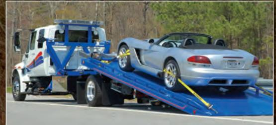
Vulcan's LCG (Low Center of Gravity) car carriers feature a deck height that's 5- to 8-inches lower, offering more stability during transport, a lower load angle and greater ease in securing loads. For recovery, Vulcan offers the SP8000 Sidepuller, the ultimate in car carrier versatility.
