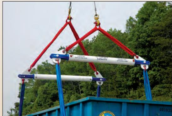
Heavy-duty recoveries require heavy-duty equipment, or at least they do most of the time. Miller Industries has developed what might be called an exception to this rule with its innovative, lightweight spreader bar.
