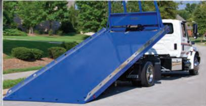
Damaged or disabled vehicles and machinery quickly unload off the LCG with its steep 20-degree dump angle.
