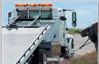
The optional SP 8000 Sidepuller provides you a multitude of recovery options that you can perform from either side of your carrier with minimal lane blockage.
