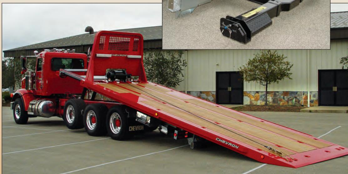
The Chevron 40 Series LCG is available in lengths ranging from 26 to 30 feet, and comes standard with a 20,000-pound planetary winch. An optional 30,000-pound, two-speed winch package
