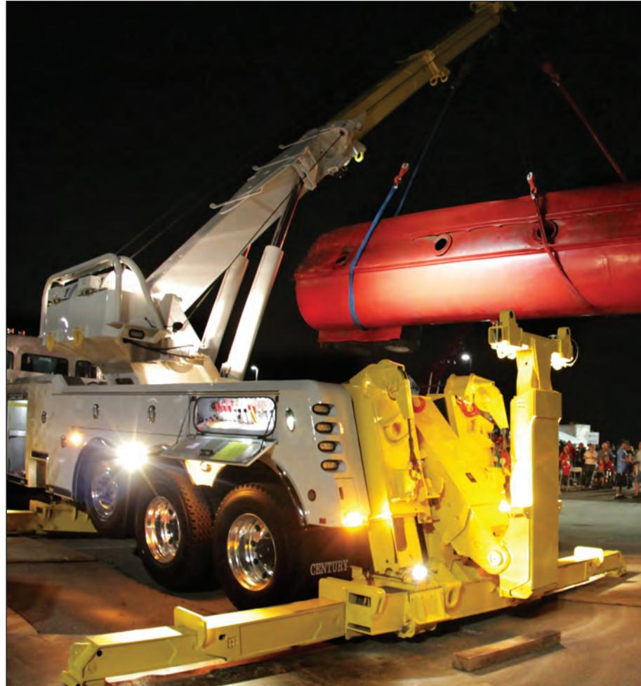
*The rear H beam outrigger option provides the operator with the same 265-inch stance as found on the front outriggers for increased stability during heavy lifting on the 1060 and 1075 rotators.*
