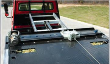
The side-mounted winch option allows you to easily adjust the cable pulley to maintain a straight-line pull on the tow eyes that have become popular on many automobiles.
