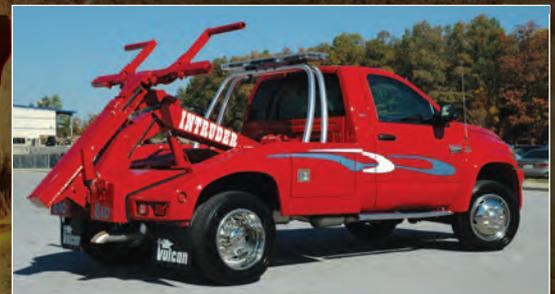
The Vulcan Intruder leads the light-duty line-up with an autoloader crossbar capable of picking up vehicles at a 90-degree angle and your choice of steel, aluminum or composite modular bodies. Other popular Vulcan light-duty units feature Vulcan's strapless wheel-lift system.
