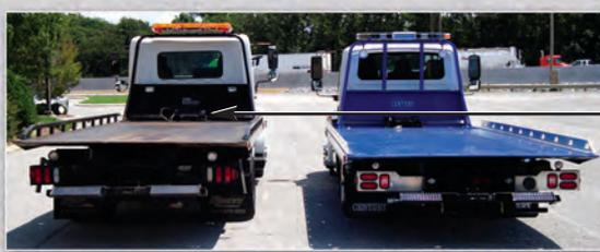
With 5 to 6 inches of lower deck height compared to a conventional carrier, the LCG provides better stability when driving down the road loaded as well as improved height clearance when hauling taller loads or operating under many lower awnings or in garages.
