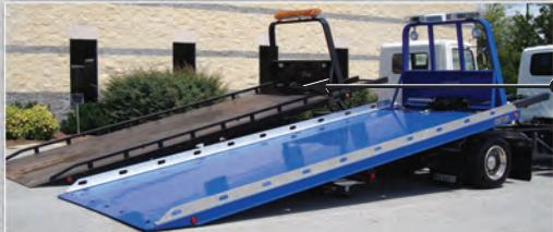
The low deck height makes it easy for the operator to reach when attaching the front tie-down chains or straps with the bed slid back and tilted compared to conventional carriers.
