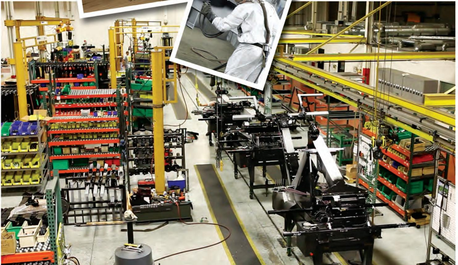
*Skilled technicians assemble and test individual components, such as recovery booms and underlifts, before installing them on the unit during final assembly. The completed unit is then tested again and given a final quality inspection.*
