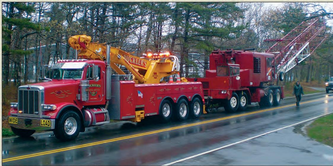
Buckler's recently responded to a call to relocate an older 80-ton-capacity Manitowoc crane in the rain, a job that was ideal for Buckler's somewhat compact Rotator. "With my boom swung forward," explained Nathan, "I have no issues with maintaining front axle weight on my truck, even when towing oversized loads in inclement weather. The versatility for both towing and recovery is just one of the many reasons we chose Century."
