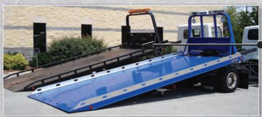
The low deck height makes it easy for the operator to reach when attaching the front tie-down chains or straps with the bed slid back and tilted compared to conventional carriers.
