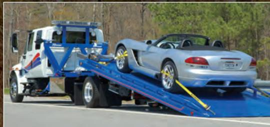
Vulcan's LCG (Low Center of Gravity) car carriers feature a deck height that's 5- to 8-inches lower, offering more stability during transport, a lower load angle and greater ease in securing loads. For recovery, Vulcan offers the SP8000 Sidepuller, the ultimate in car carrier versatility.
