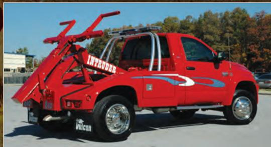
The Vulcan Intruder leads the light-duty line-up with an autoload crossbar capable of picking up vehicles at a 90-degree angle and your choice of steel, aluminum or composite modular bodies. Other popular Vulcan light-duty units feature Vulcan's strapless wheel-lift system.
