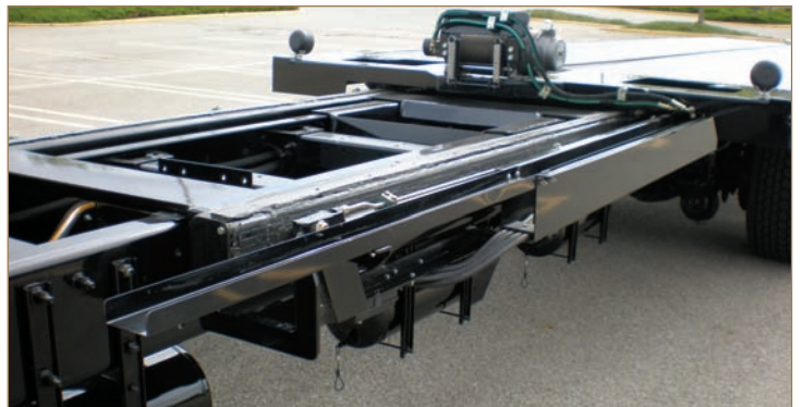
The unique patent-pending design utilizes twin slide cylinders that are mounted to a heavy-duty subframe mounted outboard of the chassis frame to achieve the low deck height.
