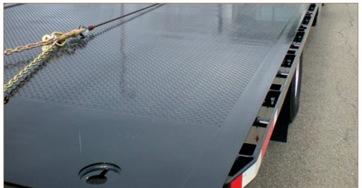
The Low Center of Gravity Carrier reduces the overall deck height of the carrier, providing better stability when hauling heavy loads as well as additional clearance for many taller loads.
