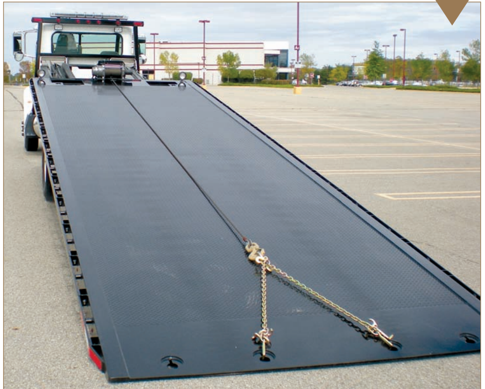
The low-mount design provides a low angle for easy loading and unloading of equipment.
