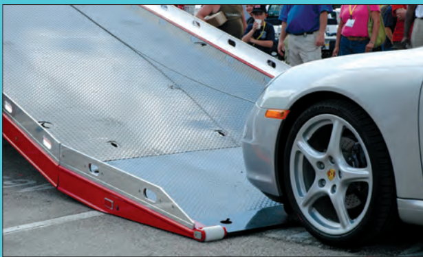
It wasn't all just heavy-duty demonstrations. A new Porsche is shown being loaded onto a new Century Right Approach Carrier with the side mount winch package and removable side rails.
