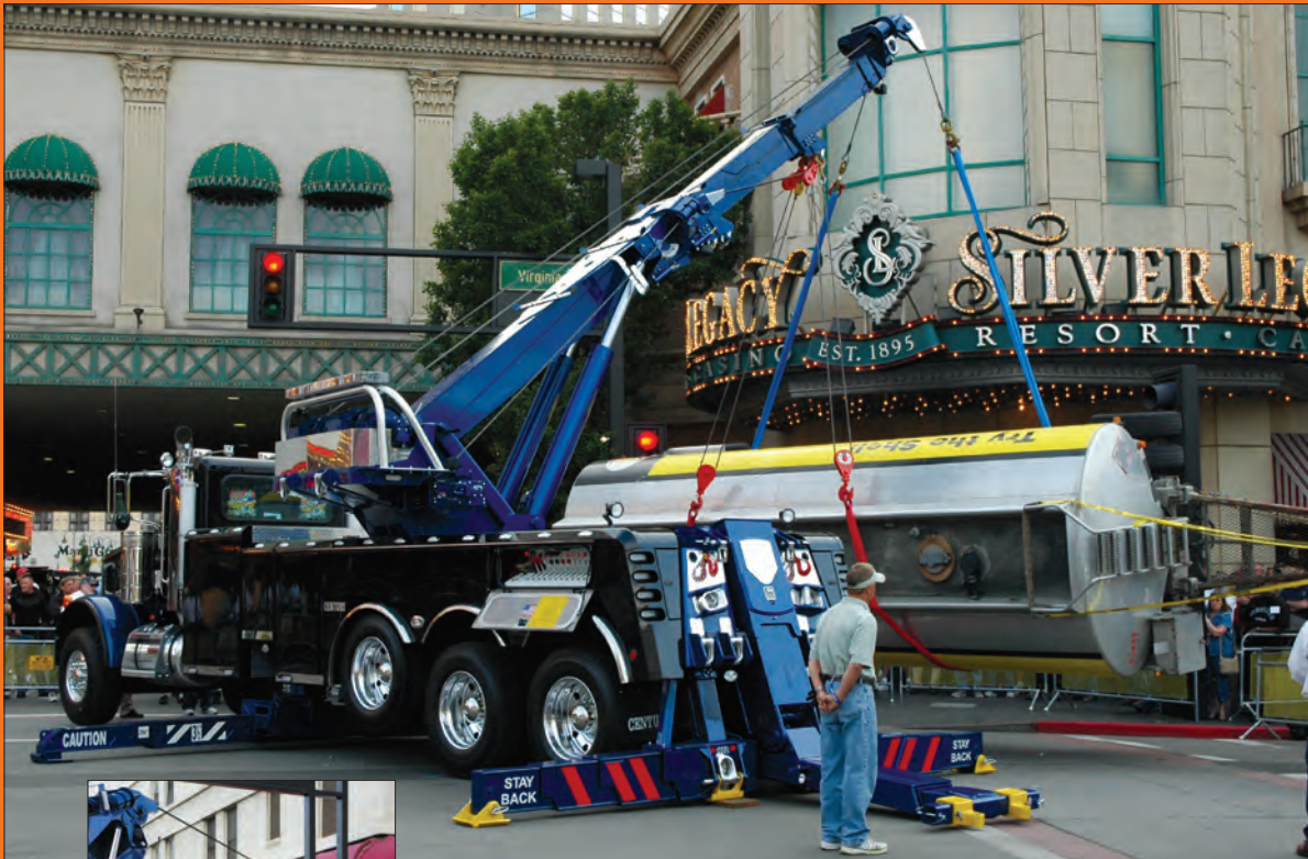
Tom John Jr. of Tom John Towing in Sun Valley, California, lifts a gas tanker, rotates it to the opposite side and barrel rolls it in the air with a new Century 1060S rotator during one of the evening's demonstrations.
