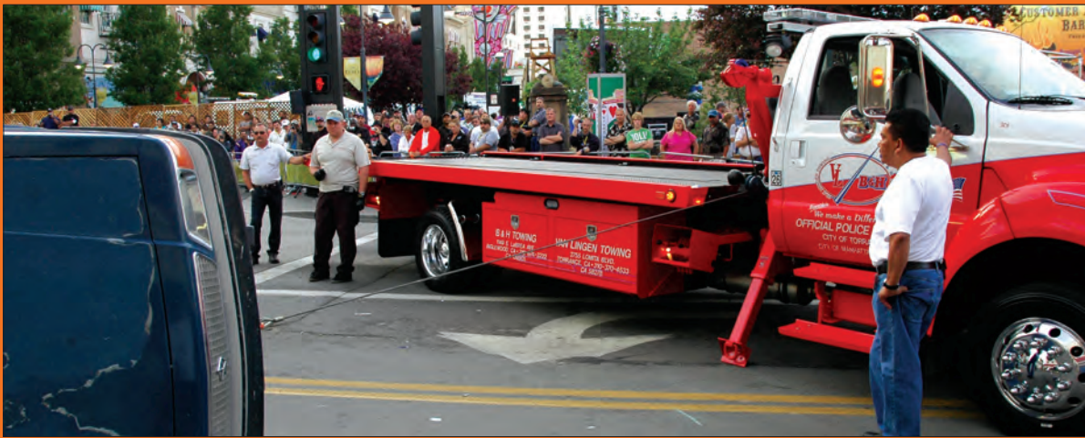
Rob Van Lingen of Van Lingen Towing in Torrence, California, demonstrates the versatility of his carrier as he recovers and rights an automobile using the SP8000 SidePuller.
