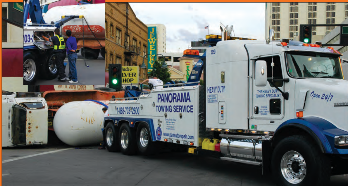
An overturned truck is righted by using the underlift to do a reverse roll while the recovery winch was used as a catch line to gently lower the casualty back down on its tires. Several recovery specialists from Panorama Towing Service in Newhall, California, used their new Vulcan V-70 to execute this recovery.
