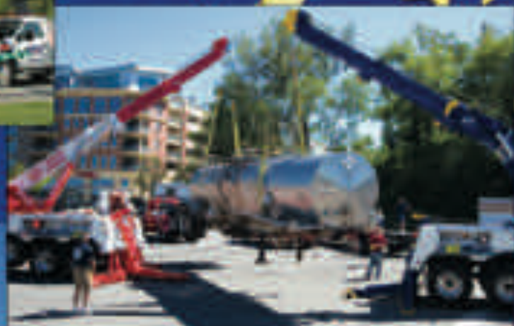
Operators display their skills as they rotate the booms to swing the tanker between the two cranes, then set it down on the opposite side.
