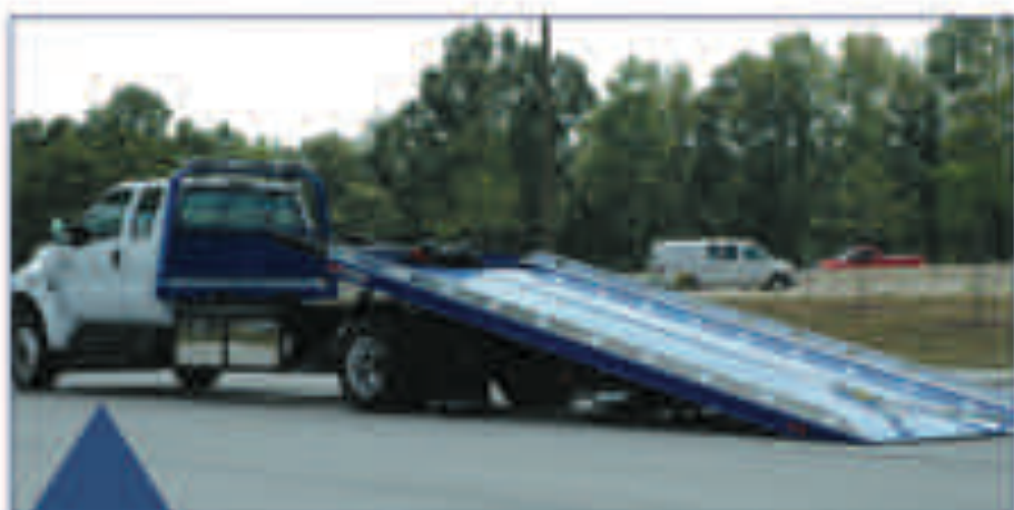
The extended subframe and mounting frame system, currently popular on Century 400 Series carriers, provides approximately 17 to 19 inches of additional maximum payload. Check it out.
