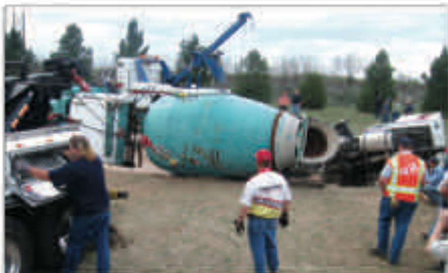
The driver's door opened this, helping decrease the resistance of the rear corner skids into the bank. The 6 ft x 6 ft block under the ladder also created a stop, helping transfer resistance.
