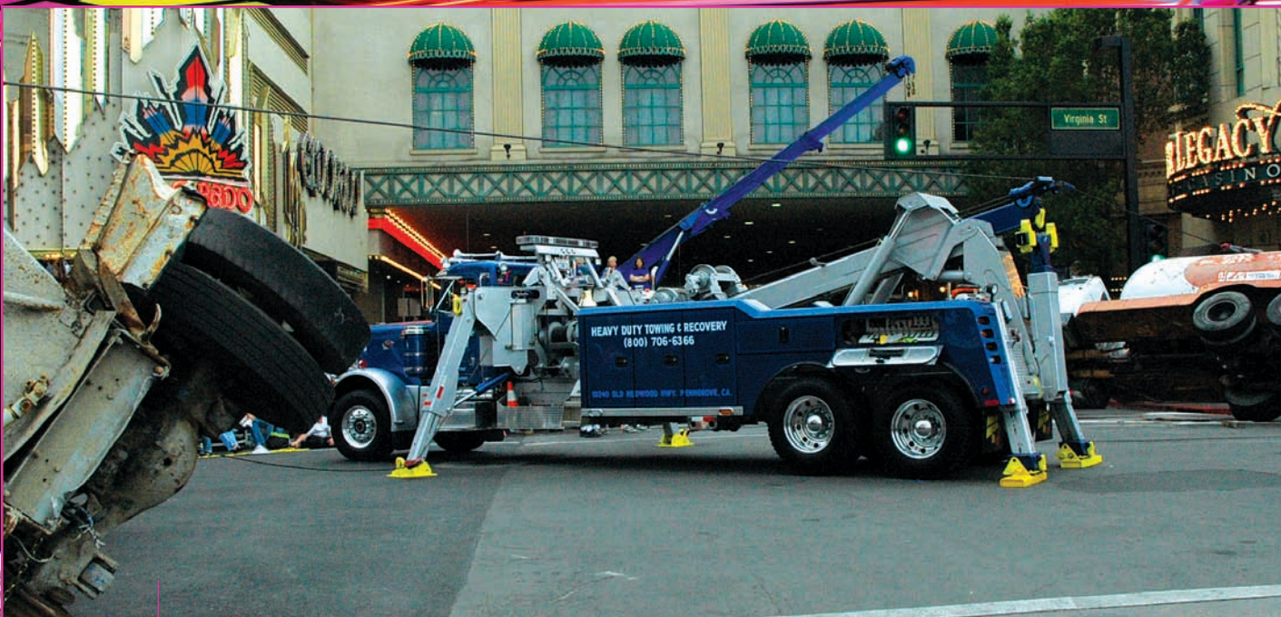
With an overturned cement mixer on one side of the intersection and an overturned propane truck on the other, a Century 7035 equipped with a SP 850 XP SidePuller, belonging to Reliance Towing Inc. of Cotati, California, rolled into the center of the intersection and was rigged to quickly right both vehicles simultaneously, showing the equipment's power and side pulling versatility.
