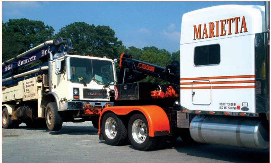
The Holmes DTU units are easy to operate and ideal for tractor swap outs, plus you can easily tow a variety of vehicles including vans, tankers and even packers.
