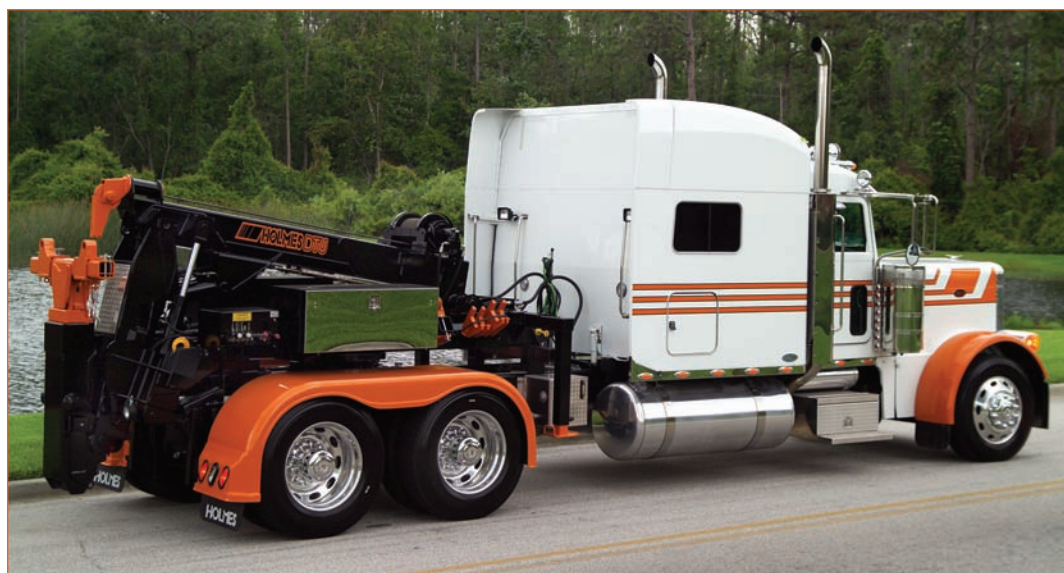
Marietta Wrecker's fleet quickly grew to include a pair of Peterbilt tractors equipped with Holmes Detachable Towing Units (DTU). The DTUs have added versatility in towing and the ability to quickly convert tractors for a variety of other uses.
