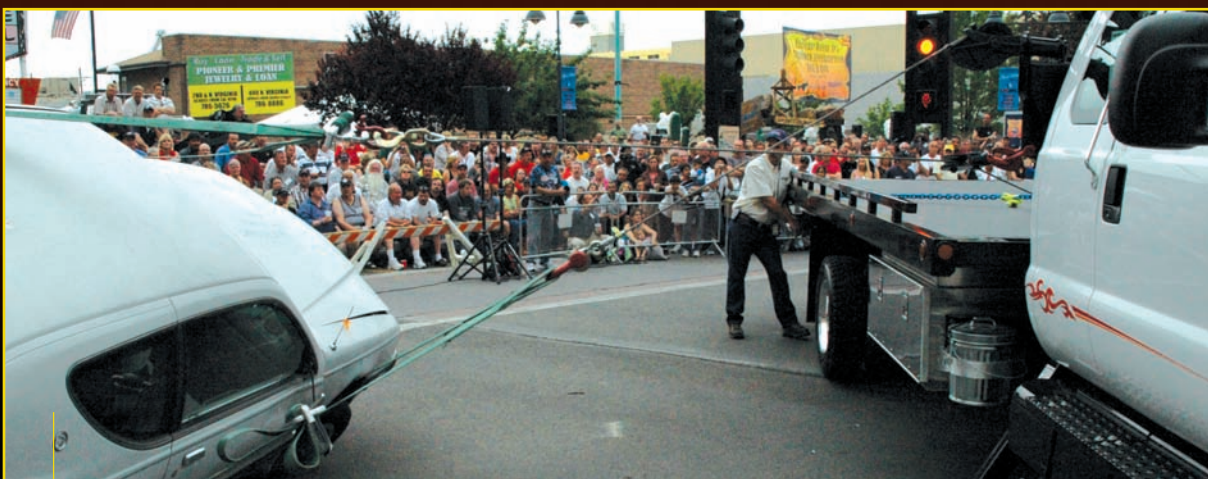
The evening's recovery began with Chuck Ceccarelli, a Certified WreckMaster instructor and inventor of the SP8000 SidePuller, removing a car that was wedged onto an overturned propane truck. Chuck used a Chevron 21-foot steel carrier equipped with a SP8000 SidePuller to perform the tricky recovery.
