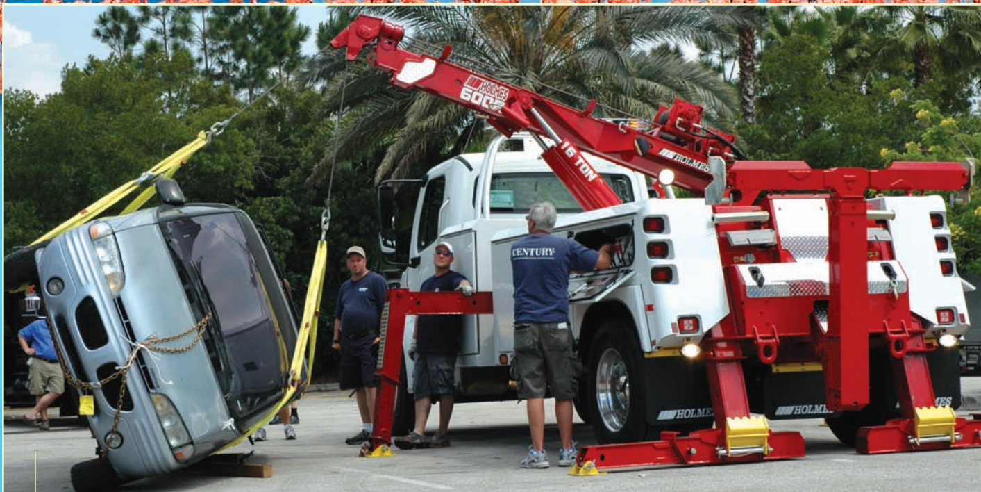
The Holmes 600R 16-ton rotator introduced at last year's Florida Tow Show demonstrated its versatility as it uprighted and lifted a van off its side.
