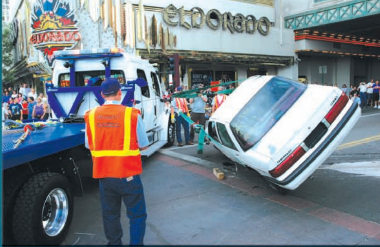
An operator demonstrates the recovery capability that can be added to a carrier by equipping it with the SP8000 SidePuller. In this staged scenario, the SidePuller is removing a vehicle hung up on a simulated guardrail.
