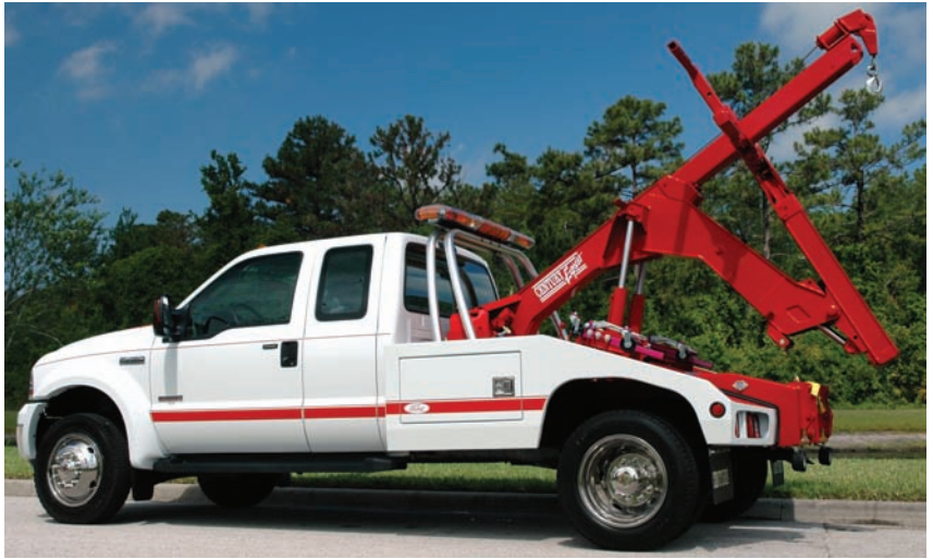
The newly introduced Century Express and Vulcan 807 are stronger yet lighter due to the use of high-tensile steel booms.
