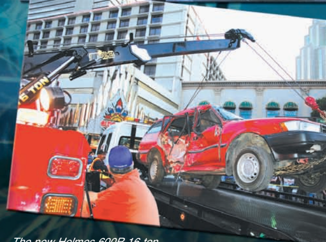
The new Holmes 600R 16-ton rotator recovers the vehicle that was crushed under the propane tank and rotates the load on to a waiting carrier to be transported.
