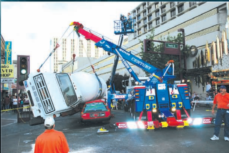
Cal-Nevada's new Century 1060S rotator performs a reverse roll on an overturned propane truck.
