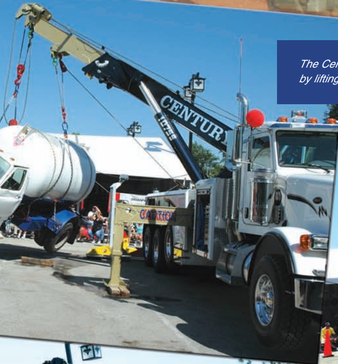
Difficult recoveries are no problem for this Century Carrier equipped with a SP8000 Sidepuller
