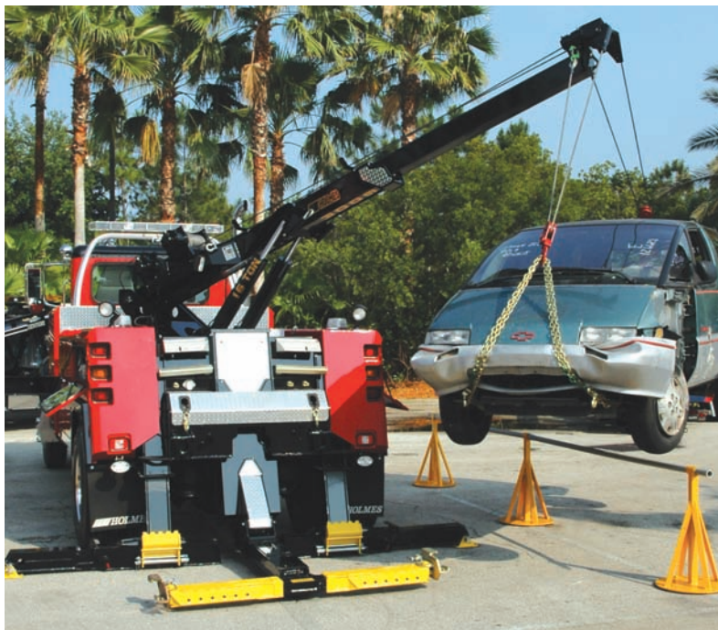
In a demonstration held at the Florida Tow Show, the Holmes 600R with its 8,500 lb. extended boom capacity easily lifts a van over a bar set up to represent a guardrail.
