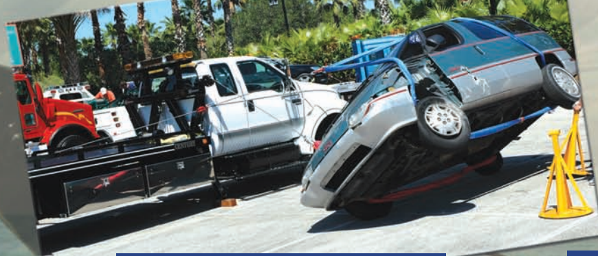
Difficult recoveries are no problem for this Century Carrier equipped with a SP8000 Sidepuller
