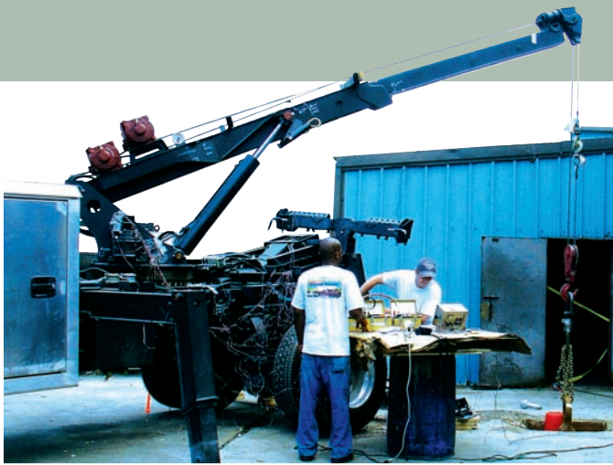
After completing computer simulated stress and finite analysis, a prototype unit is built. Miller Industries' engineering staff then conduct rigorous strain gauge tests to ensure the unit will perform to their tough standards.
