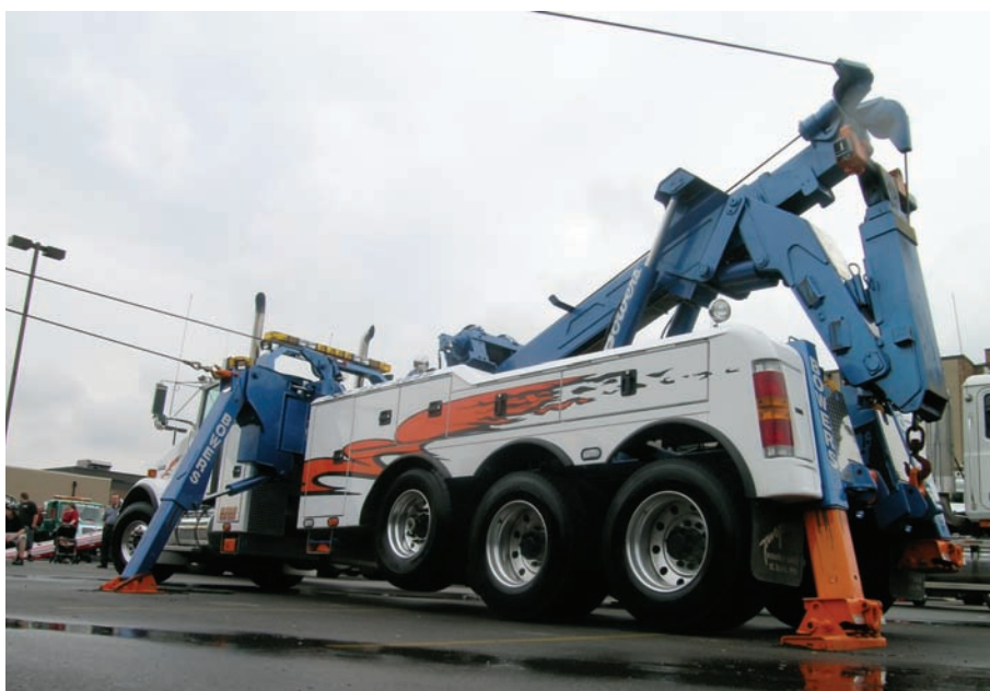
For a typical heavy side pull operation, the front winch line on the SP-850 XP is run through a snatch block at the casualty and then attached back at the D-ring located on the top of the jackleg. One line from the main winch on the recovery boom is run to the casualty and the opposite winch line is run down to the rear tailboard D-ring to help stabilize the boom.
