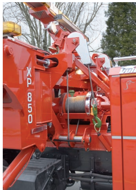
The XP's winches are mounted low into the frame with the cable running through a pulley and up through a pivoting sheave head. This system, which includes an air tensioner, provides for better cable spooling while allowing repositioning of the jack leg without affecting the winch line.
