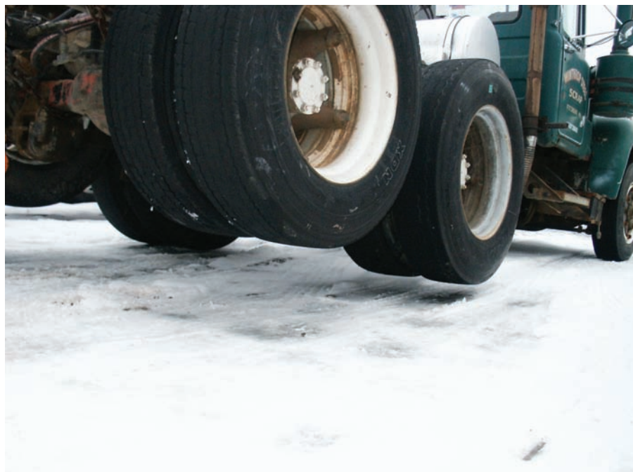
Lifting the rear axle using forks can cause problems by having to raise the vehicle to an excessive height.
