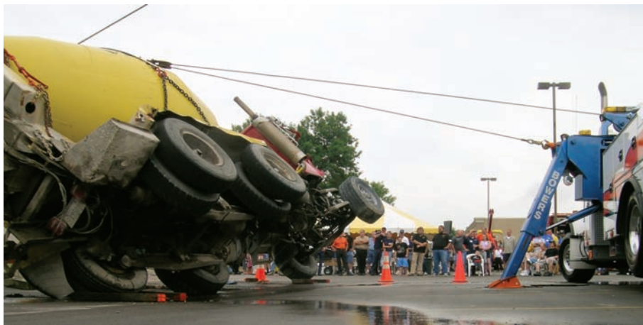
The SP-850 XP allows the operator to perform recoveries off the side, ideal for narrow roads or when trying to minimize lane closures. This capability is reminiscent of the older Holmes mechanical wreckers.
