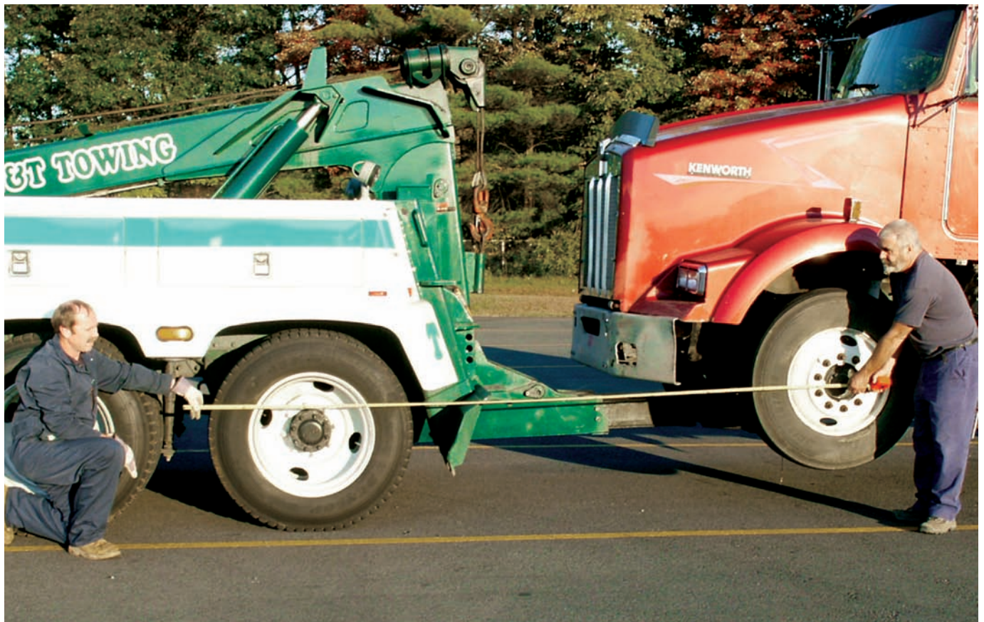
The overhang is measured from the trunnion (center point between the two axles) to the lift point on our towed vehicle, which in this hookup is the front axle.
