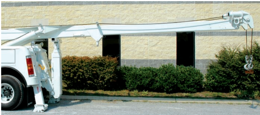
Challenger's independent boom and underlift allows for the boom to travel back and forth without interference from the underlift at any boom elevation.
