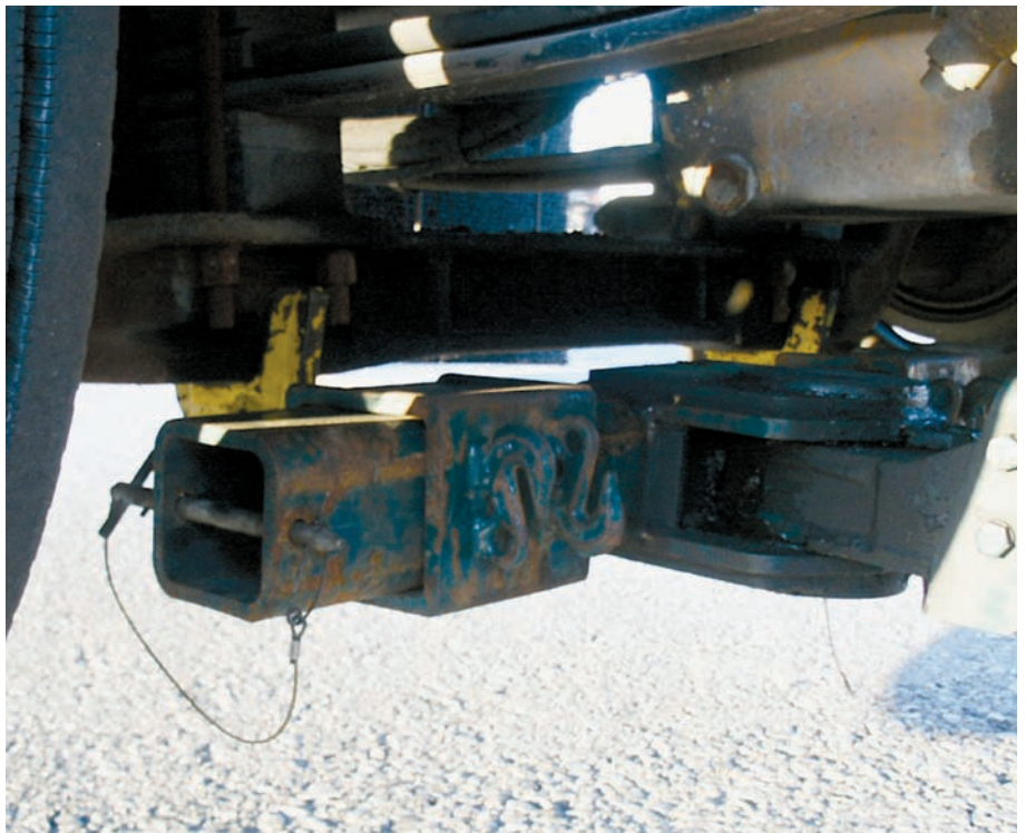
Lifting the truck at the steer axle using a set of 3-inch, short lift forks is one of the most common hookups used today.
