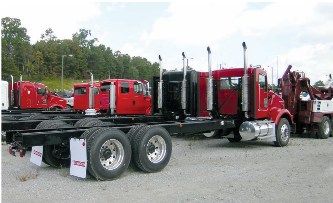
The chassis are ordered with the correct frame lengths and RBM rating so frame stretching or additional reinforcement is not necessary. Outside frame rails behind the cab are clear of air and fuel tanks, and air and electrical hook-ups are located at the rear of the frame.
