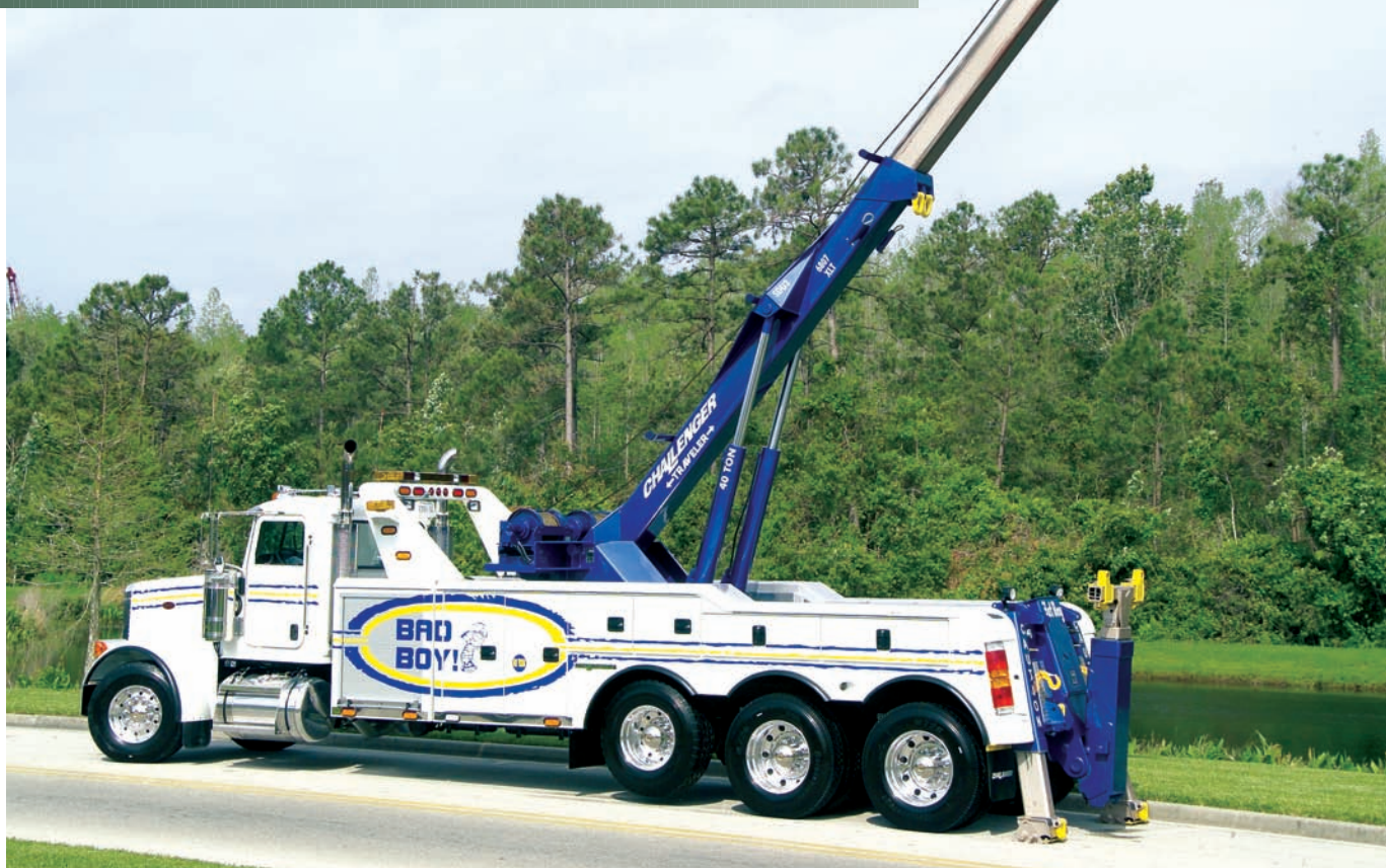
The Challenger XLT Series two-stage boom extends 156" for more power and capacity. The boom can travel 72" backward or forward with a suspended load at 60 percent of its rated capacity.
