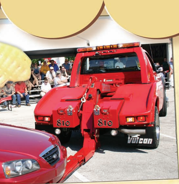
Paul Craze of Miller Industries demonstrates how easily the Vulcan Intruder with the new composite body can hook up to a vehicle at a 90° angle.
