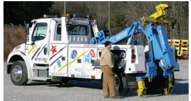
A Century 3212 is positioned as a catch truck to hold the mixer as it comes over.
