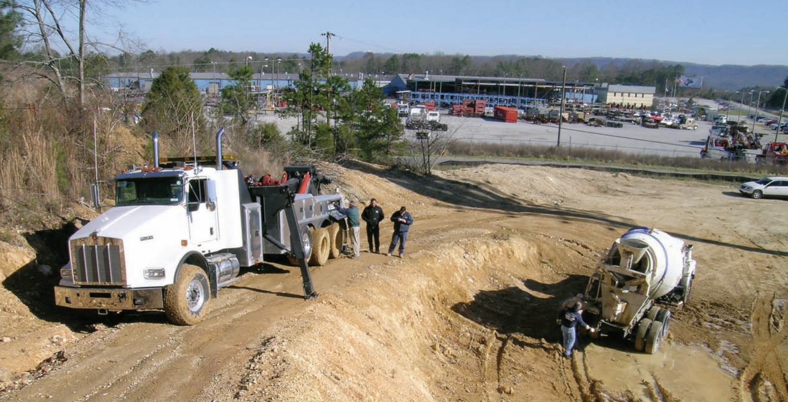
The Century 9055 SP850XP is rigged to the mixer mired in the mud below.
