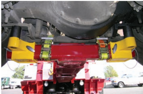
The U-bolt attachments lift the tractor by the axle saddles. Chains or tie-down straps are installed to secure the vehicle to the cross bar.
