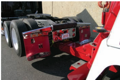
The U-bolt attachments are ideal for hard-to-tow tractors with chrome dress up kits and custom light packages.
