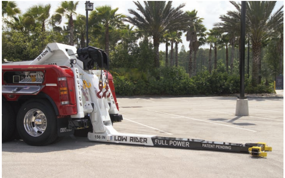
The U-bolt attachments lift the tractor by the axle saddles. Chains or tie-down straps are installed to secure the vehicle to the cross bar.
