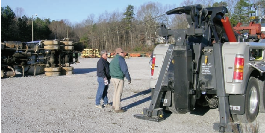
Lines are rigged from the Century 9055 SP850XP to the tipped mixer.
