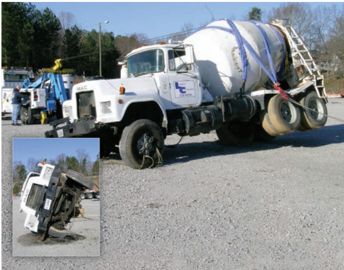
Lines are rigged from the Century 9055 SP850XP to the tipped mixer.
