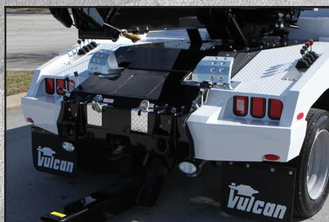
Vulcan light-duty conventional units come standard with tailboard D-Rings, wheel retainer storage pockets and separate boom and wheel lift controls for more versatility and ease of use.
