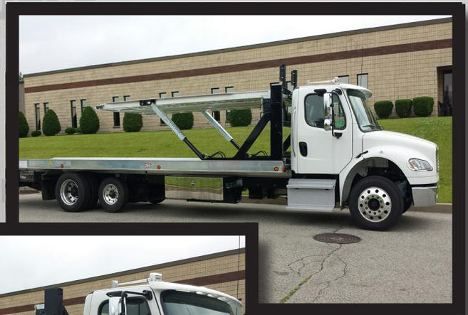
The upper deck lowers flat onto the bottom deck to allow the operator to easily load and secure the vehicle without climbing onto the truck or deck.
