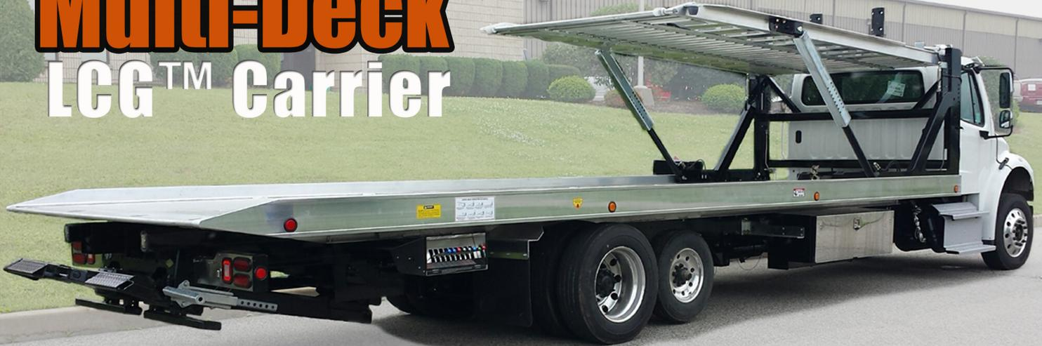
**The combination of proven technology and reliability of a 16 Series Aluminum LCG™ (Low Center of Gravity) Carrier with an auxiliary deck system. The Multi-Deck Carrier is available in deck lengths from 24-26 feet for hauling up to 3 vehicles as well as 30 foot decks for transporting up to 4 vehicles.**
