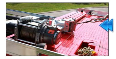
The optional SlideWinder planetary winch allows the operator to easily adjust the roller guide position to maintain a straight pull on the vehicle when using a screw in tow eye that are popular on many cars.
