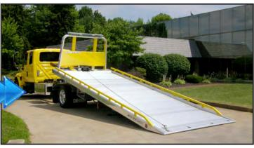
The LoadRite II on steel decks provide bi-directional chain locks every 12" down the inside rail allowing the operator to quickly and easily secure vehicles with almost any type of tie down systems.
