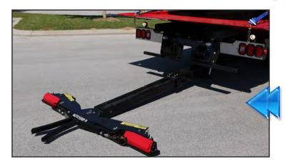
To provide quick and easy hook ups without the hassle of L Arms for towing a second vehicle, your LoadRite II can be equipped with the AutoGrip II wheel lift.
