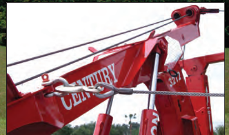
The 3212 G2 allows the cable to be run through a snatch block and hooked to a clevis at the base end of the boom for side pull applications.
