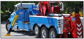
The Century RXP option for the 1140 tri-axle rotator incorporates dual 35,000-lb., two-speed planetary winches, as well as 212" of spread for more stability.
