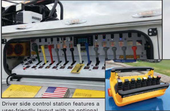
Driver side control station features a user-friendly layout with an optional wireless remote to allow you move to an optimal vantage point.
