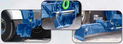
Independent rear spades provide a wide foot-print and are available with optional multi-position flipper feet or extendable rear outriggers.
