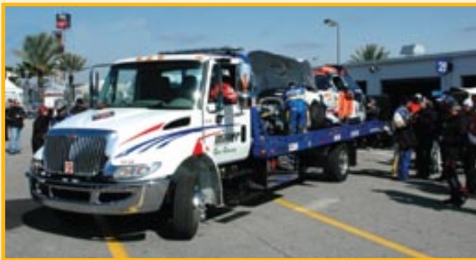
This year's fleet of Miller Industries Race Recovery vehicles included five new CENTURY® 12 Series LCG carriers. The new lower deck height and low load angle were beneficial for loading race cars providing the same advantages many towing companies have already discovered in the LCG carriers in their fleets.
