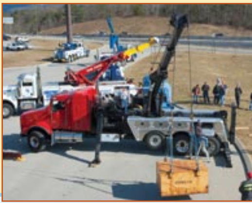
◀ A Century 1140 rotator with the new RXP pivoting front stabilizer legs lifted a 20,000-lb test weight and then rotated it from one side of the truck to the other. Meanwhile, in preparation for the next demonstration, a Century 1060S rotator was already positioned behind the 1140 and hooked up to a loaded mixer drum weighing 44,000 lbs.
