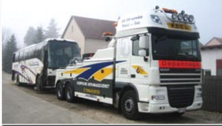
A DAF chassis equipped with a CENTURY® 9055 proves to be a rugged workhorse for serious truck wrecks and recoveries. The low profile and long reach of the 9055's underlift make it ideal for towing buses and coaches that are very common in Europe.
