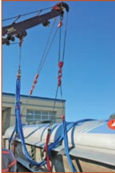
▲ A Century 1140 rotator performed a reverse roll on a loaded tanker. As the tanker comes over, you can see how it's controlled with the catch line on the high side. You can also see how the traveling snatch blocks hooked to the continuous loop straps help spread out lift points on the loaded trailer. We've found that the slings that work best with traveling blocks are 3/4-inch wire rope, 12-foot long with a wire rope eye on each end.
