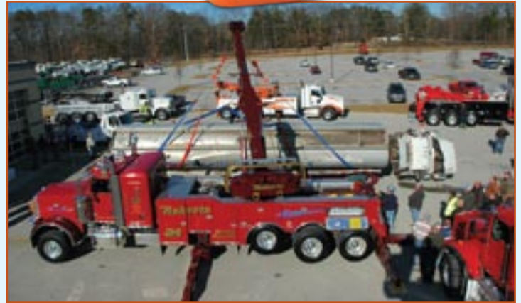
▲ A Century 1140 rotator performed a reverse roll on a loaded tanker. As the tanker comes over, you can see how it's controlled with the catch line on the high side. You can also see how the traveling snatch blocks hooked to the continuous loop straps help spread out lift points on the loaded trailer. We've found that the slings that work best with traveling blocks are 3/4-inch wire rope, 12-foot long with a wire rope eye on each end.
