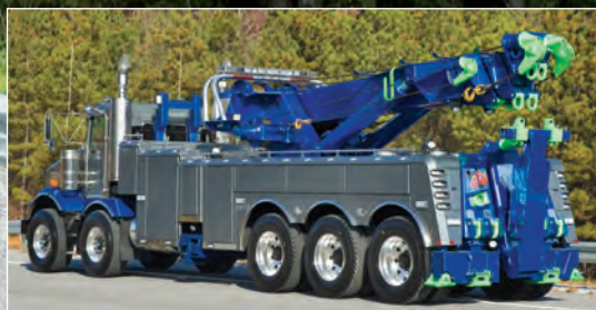
To tackle your most difficult recovery jobs for heavy loads, rely on the brute strength of the Century 1075S (75-ton), equipped with a 3-stage recovery boom and available with up to 6 winches for a combined winching capacity of 234,000 lbs.
