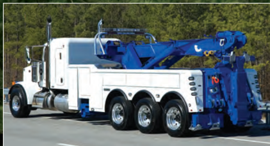
The Century 1140 (40-ton) rotator fits most applications, with options such as a 2- or 3-stage recovery boom, dual 35,000-lb. 2-speed winches, LDU underlift and a combination of auxiliary winch and outrigger systems.
