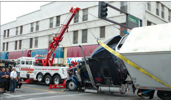
A CENTURY® 1140 (40-ton rotator) and a CENTURY® 9055 demonstrate an in-line roll of an overturned tractor and trailer on the narrow streets of downtown Reno.
