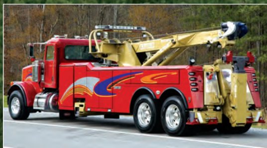
The Century 1130 (30-ton) rotator provides the versatility of a rotator for recovery applications with a weight-conscious design for increased towing payload.
