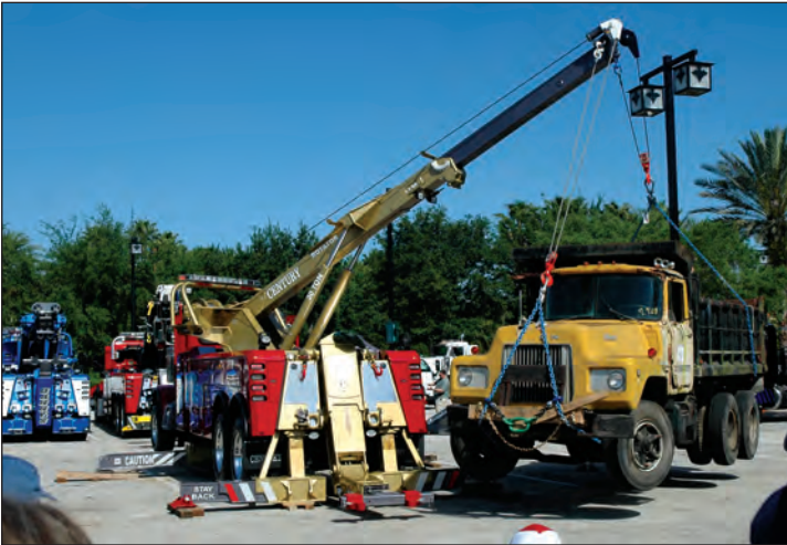
The newest member of the CENTURY® family of rotators, the 1130 (30-ton) lifts and rotates a tandem dump truck around the rear of the unit during one of the demonstrations at the Florida Tow Show®.
