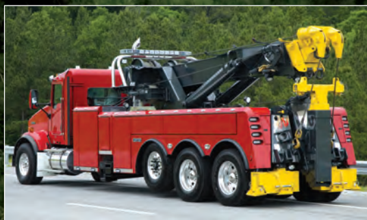
The Century 1060S (60-ton) provides 360-degree continuous boom rotation, a 3-stage recovery boom, optional turret-mounted and deck-mounted winches, your choice of outrigger package, and the proven SDU-4 underlift.
