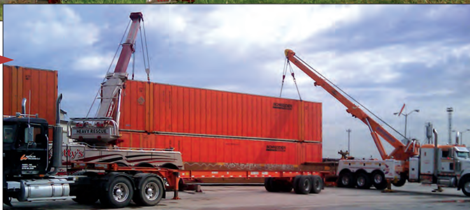
Scotty's CENTURY® 1075S, working with a CENTURY® 1075S Rotator from Independence Towing in Kansas City, lifts loaded rail containers onto waiting trucks.
