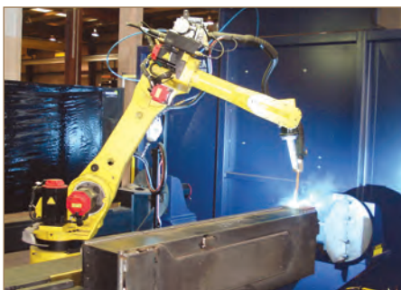
One of the two new robotic welders in the heavy-duty department provides a smooth consistent weld on an underlift boom.
