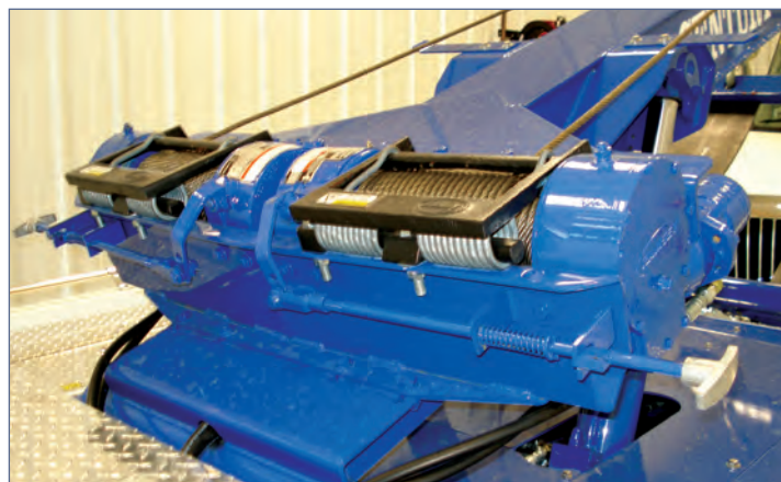
On the new four-plate fabricated recovery boom, the winches are mounted at the base of the boom above the pivot. This allows the boom to be raised and lowered without affecting the cable moving in relation to the cable guides, the same as on most integrated units. Cable tensioners and winch clutch releases are standard equipment.
