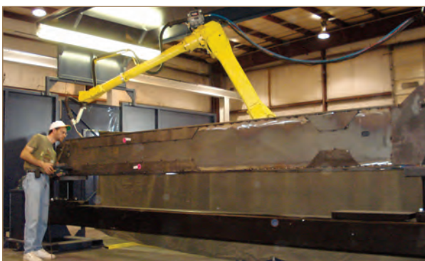
A Miller Industries technician programs the new large robotic welder to weld an outer boom for a Century 1075S rotator.
