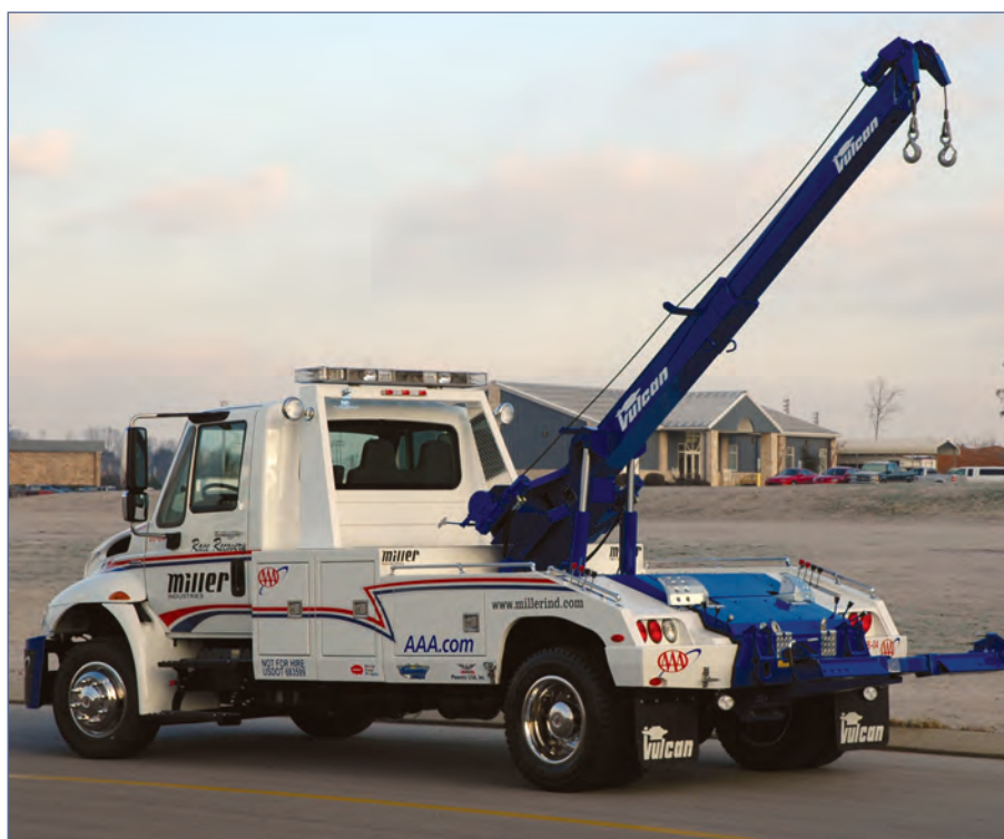
The Vulcan 892 and 894 designs provide for increased lifting height with the new fabricated recovery boom. A new modular carbon steel body with optional front tunnel boxes is available as shown on this Vulcan model 892.
