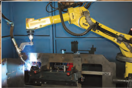
A robotic welder provides fast, efficient and consistent quality welds to the carrier's components.
