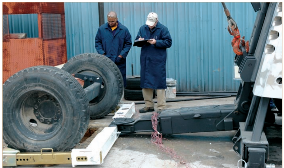
Engineers prepare the new 25K wheel-lift for testing utilizing strain gauges and a load cell.
