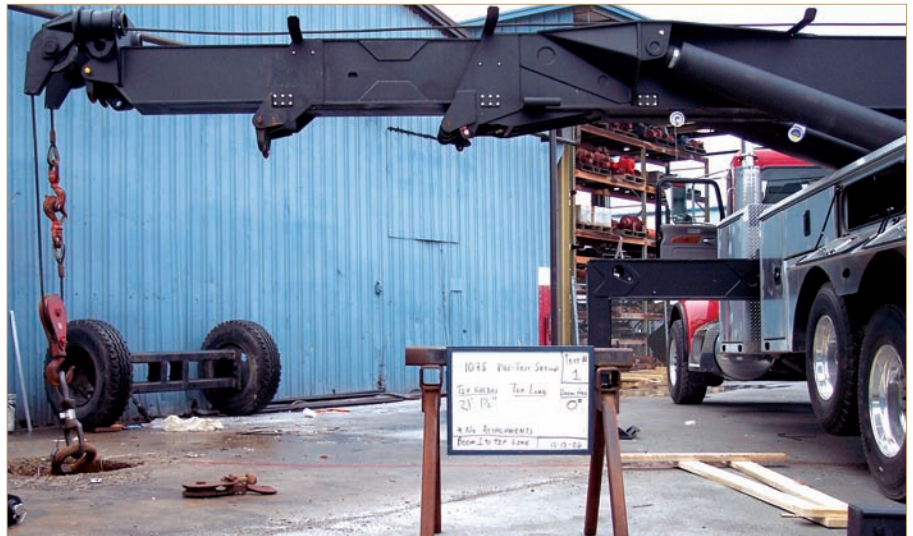
After completing simulations, the 1075S is rigged in the test pit for actual side pulls to verify the tip chart data.
