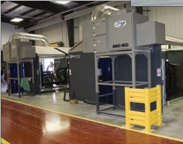
Welding cells will perform finish welding on major components such as booms and subframes.
