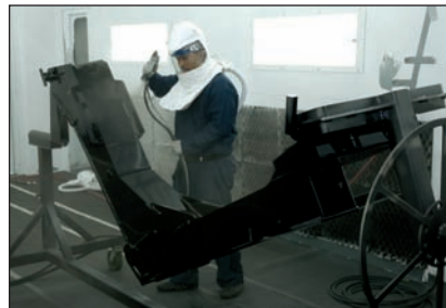
After the blast process, the cart is rolled into the paint booth where an epoxy primer and gloss urethane enamel is applied.
