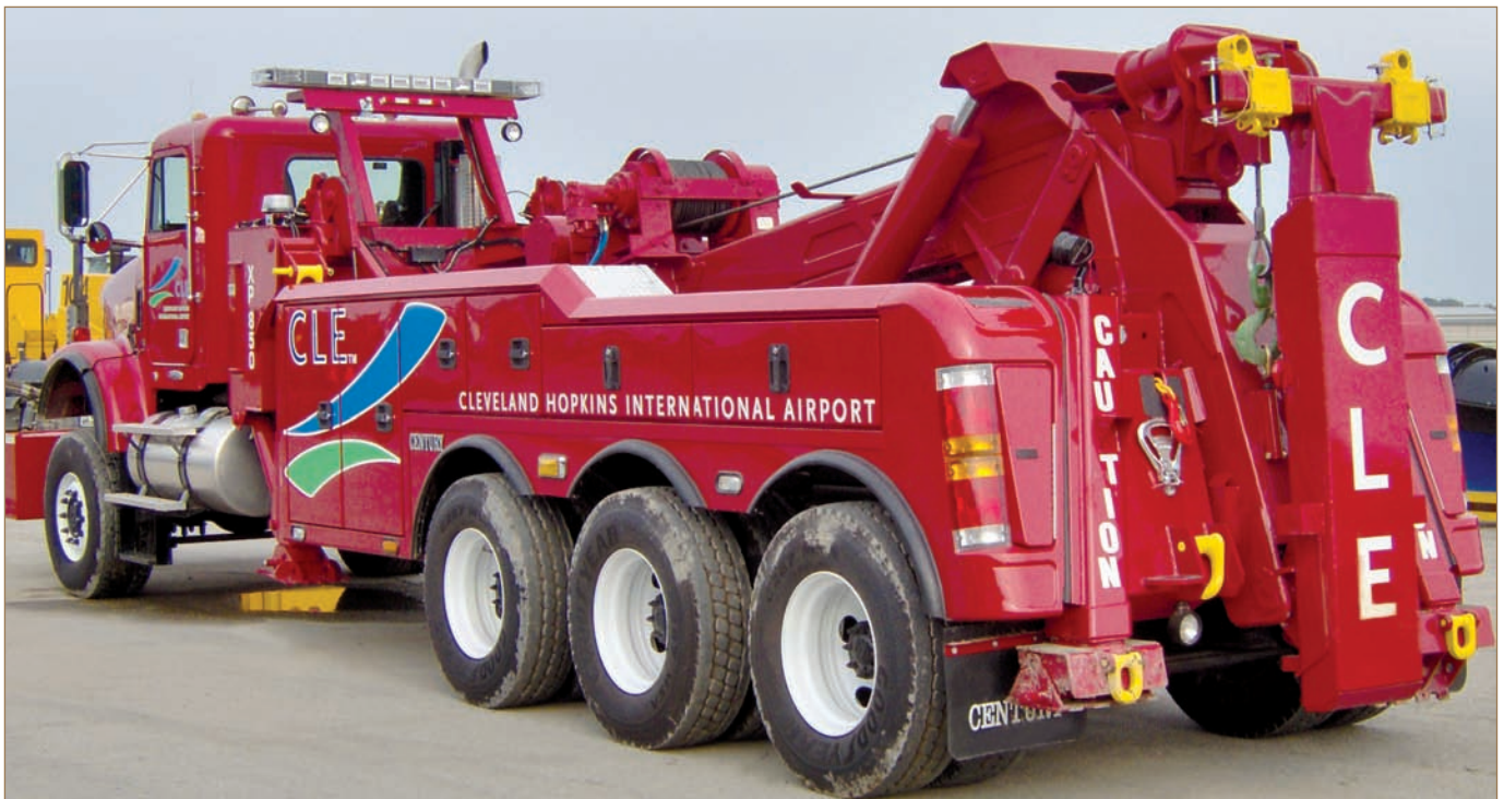
This all-wheel-drive, tri-axle Freightliner chassis with a Century 9055 SP850 XP, front winch bumper and Low Rider underlift is in service for the Cleveland Hopkins International Airport.
