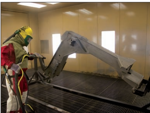
Welded components are loaded onto carts and brought through a grit blast booth to remove rust, mill scale or weld spatter from the surface for better paint adhesion.
