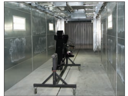
Before heading to the assembly line, the cart is pulled through a tunnel oven and cool-down area.
