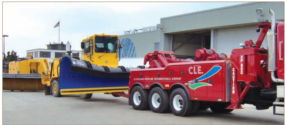
The Cleveland Hopkins International Airport has some of the most demanding airport snow conditions in the world. It is cleared by an all-wheel-drive chassis to push 25-foot plows and pull 30-foot brushes. The Low Rider's low profile enables it to get under the plow, lift 18,000-plus lbs. and safely tow the unit
