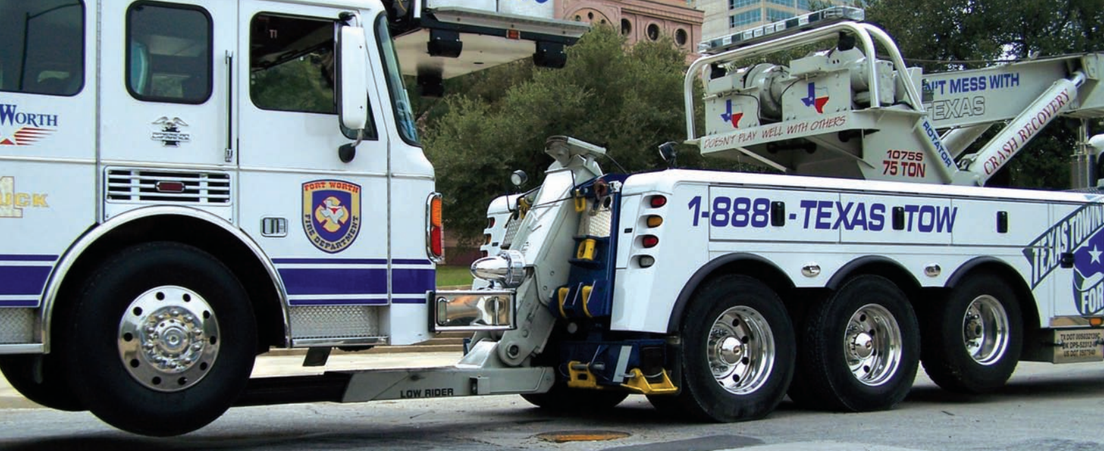
The Low Rider option provides the additional reach sometimes needed in difficult towing applications such as fire trucks with set back axles, extended front bumpers, and ladders, buckets or snorkels protruding past the front of the vehicle. The low profile of the stinger also allows for additional clearance between low hanging pumps, bumpers or oil pans.
