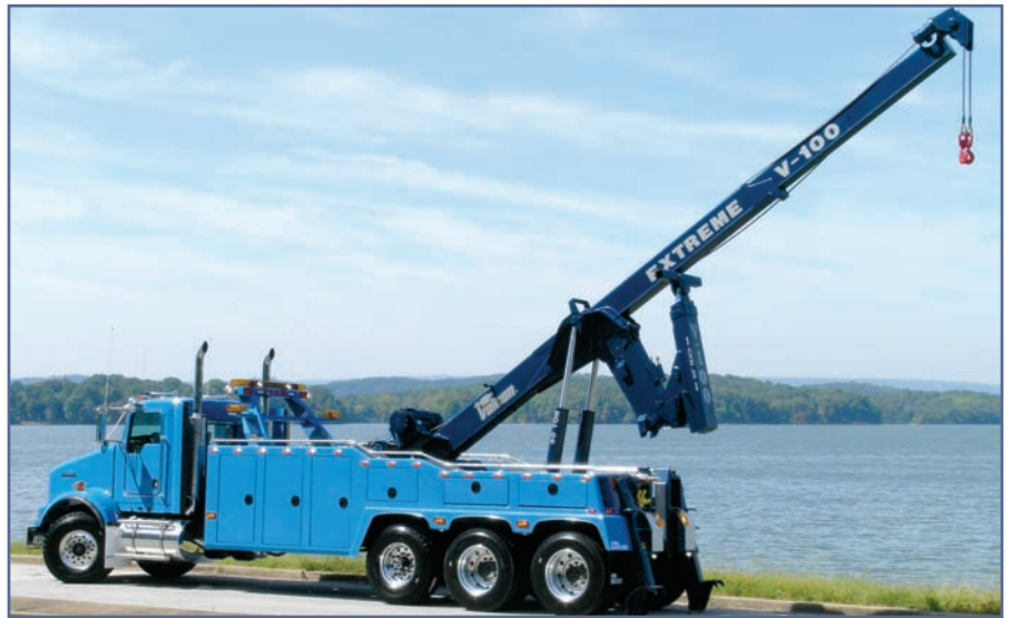
By adding a three-stage boom option to the popular Vulcan V-100 and Century 9055, these much lighter weight integrated towing and recovery units now have similar reach and recovery capabilities as conventional fixed-boom models.
