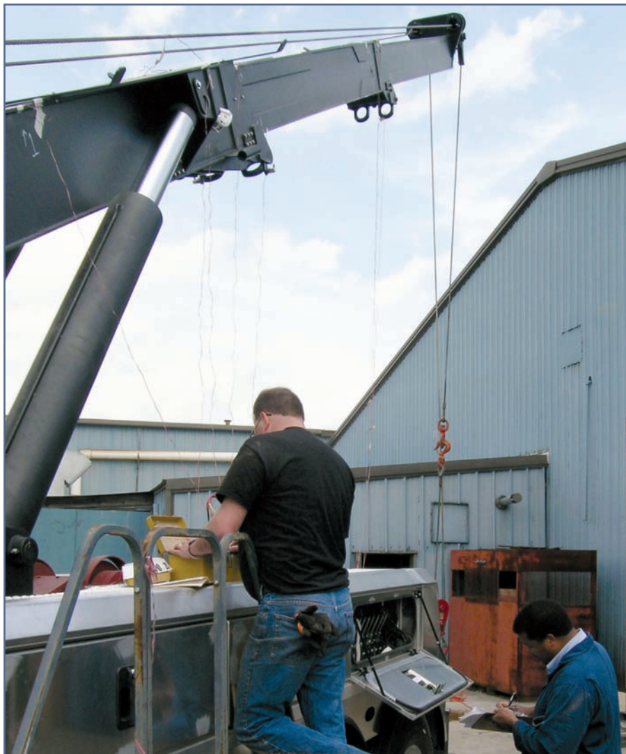
After months of design and testing using the latest Pro-Engineer 3-D CAD design software, along with performing Finite Element Analysis on the structure, Miller engineers are ready to put a prototype 75-ton rotator through the final strain gauge tests.
