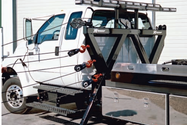
The SP8000™ is designed so the sheave head attachment can be moved easily so the operator can winch off either side of the truck. A D ring mounted on the bottom foot of the stiff leg, along with additional anchor points to accommodate shackles and snatch blocks, allow for a variety of rigging possibilities during difficult recoveries.
