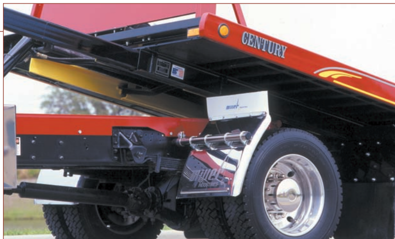
The lower mounting frame, shown in red, is found exclusively on the Century and Challenger carriers providing additional reinforcement to the chassis frame rail. A bolt-on reinforcement is provided with the Chevron, Champion and Vulcan product for many applications.
