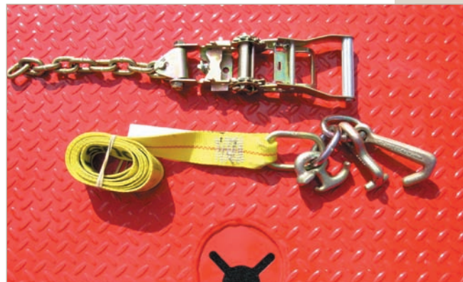
Cluster strap assembly with R hook, T hook and mini J.
